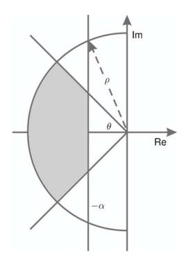
Figure 4.3: Desired pole location
