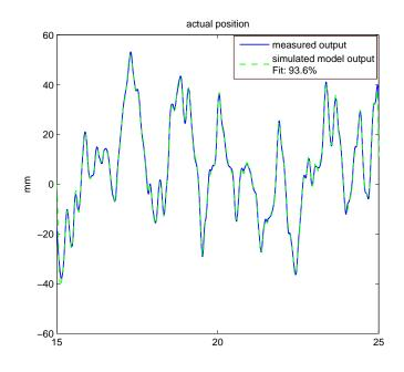
Figure 6.4: Validation of the obtained model for bottom actuator
