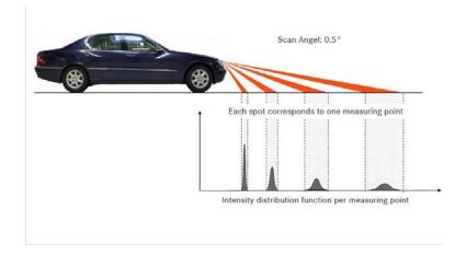
Figure 1.7: Disturbance detection scheme of ABC-Prescan [49].
