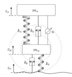
Figure 2.1: A quarter-car active suspension system
