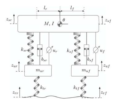
It consists of the sprung (body) mass, two unsprung masses (wheel-axle assemblies)
