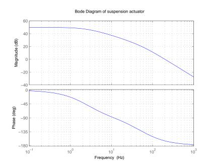
Figure 5.3: Bode diagram of the suspension actuator
