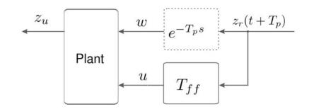
Figure 3.1: Feedforward control design scheme
