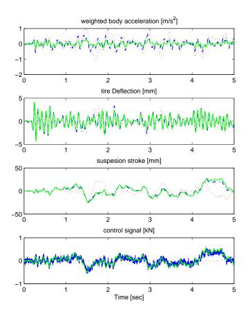
Figure 3.8: Real road response of the Multi-objective design: Preview (-), Pure feedback (-.), Passive (..)
