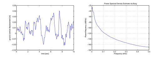
Figure 2.3: A real road profile; left: time history (ground vertical displacement), right: power spectral density corresponding to ground vertical velocity
