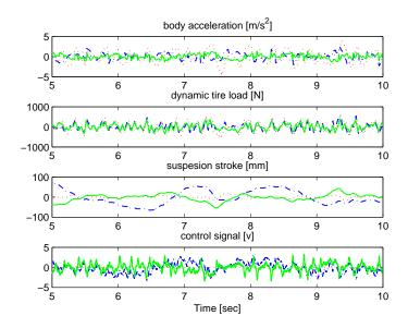
Figure 5.6: Real road response of the preview design considering actuator dynamics, based on nonlinear model simulations: multi-objective (-), LQ-based (-.), Passive (..)
