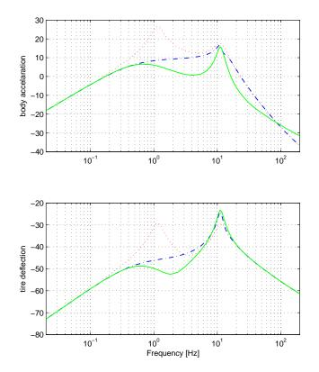
Figure 3.7: Frequency Response of the Multi-objective design: Preview (-), Pure feedback (-.), Passive (..)
