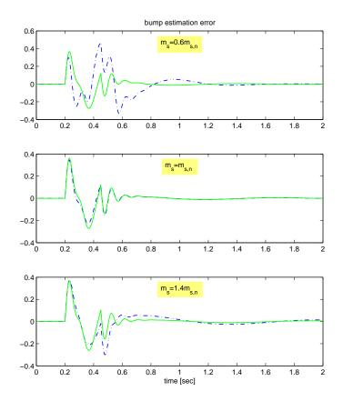
Figure 4.4: Performance of estimators for the bump input: LPV- $H_{\infty}$  (-), Kalman (-.)
