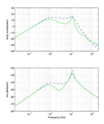
Figure 3.6: Frequency Response of the LQ-based design: Preview (–), Pure feedback (-.), Passive (..)
