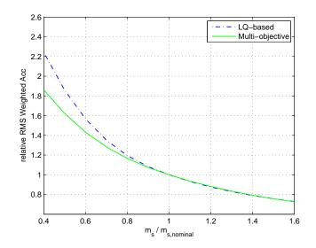
Figure 3.9: relative RMS weighted acceleration: multi-objective preview(-), LQ-based preview(-.)
