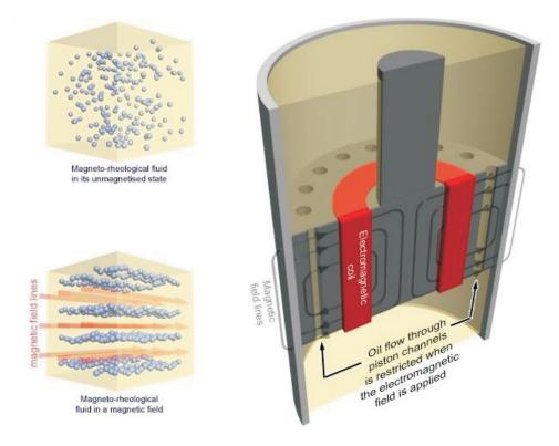
Figure 1.4: working principle of MR damper, figure from [36]
