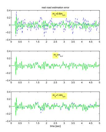
Figure 4.5: Performance of estimators for the vibration input: LPV- $H_{\infty}$  (–), Kalman (-.)
