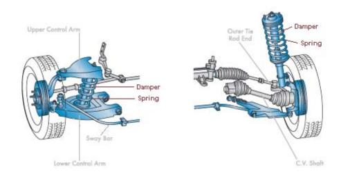
Figure 1.1: Two most common front suspension types. Left: Control arm type, Right: (McPherson) strut type. Figure from www.midas.com
