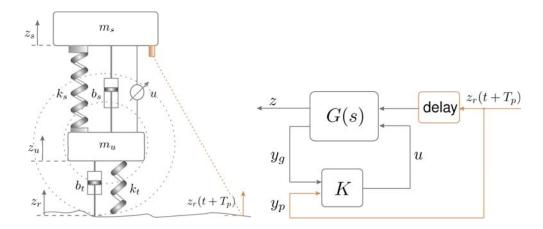
Figure 3.2: left: preview suspension concept, right: corresponding design framework
