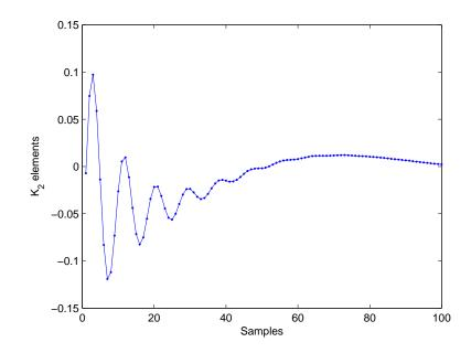
Figure 3.5: Coefficients of preview signals of different times ahead of wheel
