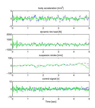
Figure 5.4: Real road response of the Multi-objective design considering actuator dynamics, based on nonlinear model simulations: Preview (-), Pure feedback (-.), Passive (..)
