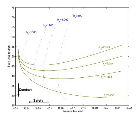
Figure 1.2: Ride comfort vs. safety for different values of the suspension elements
