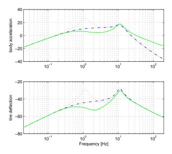
Figure 3.10: Frequency Response of the Multi-objective design with improved safety: Preview (-), Pure feedback (-.), Passive (..)
