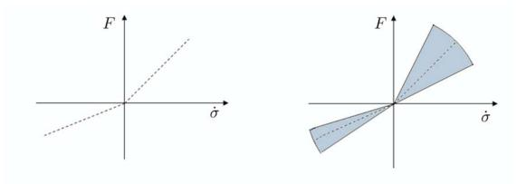
Figure 1.3: Damper characteristics, left:passive suspension, right:semi-active suspension;  $\sigma := z_s - z_u$
