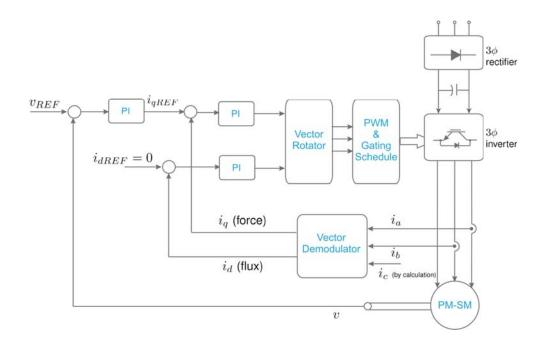
Figure 5.2: Field oriented control of a PM-SM
