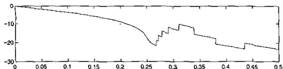
Fig. 2. Phase response (radians) of a 17th order bireciprocal wave digital filter.
