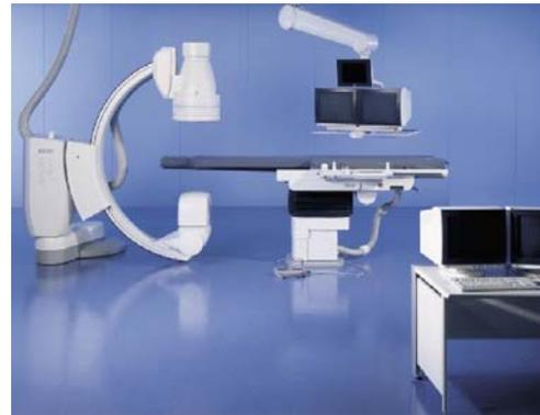
(b) floor-mounted stationary C-arm with image intensifier
