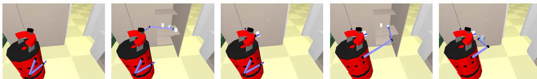
Figure 4.11 Sequence where the cupboard door is closed and opened again between taking two cups of the cupboard
