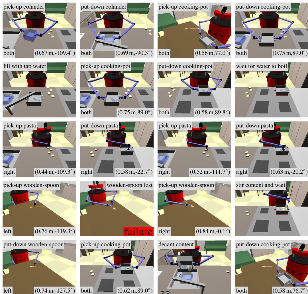
Figure 4.7 Plan for boiling pasta showing some higher-level manipulation plans as a slide show.
