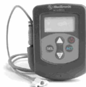
Figure 5 - CGMS System Gold minimally-invasive glucose meter from Medtronic MiniMed. The sensor is inserted under the skin on the abdomen and can monitor interstitial glucose up to 72 hours (GROSS, BODE and EINHORN, 2000).
