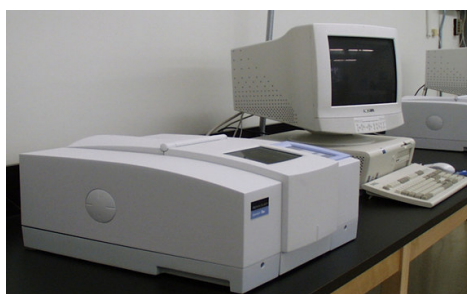
Figure 60 – FTIR spectrometer and supervision computer, this device does not require the use of reference, since it can collect background spectra of the ambient light (PERKIN-ELMER, 1998).
