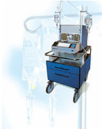
Figure 110 – Biostator artificial pancreas which is able to continuously monitor venous blood glucose.
