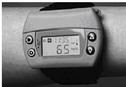
Figure 8 - GlucoWatch wrist-watch blood glucose monitor from the company Cygnus. Glucose is extracted through reverse iontophoresis, and measured by amperometric biosensor (POTTS, TAMADA and TIERNEY, 2002).
