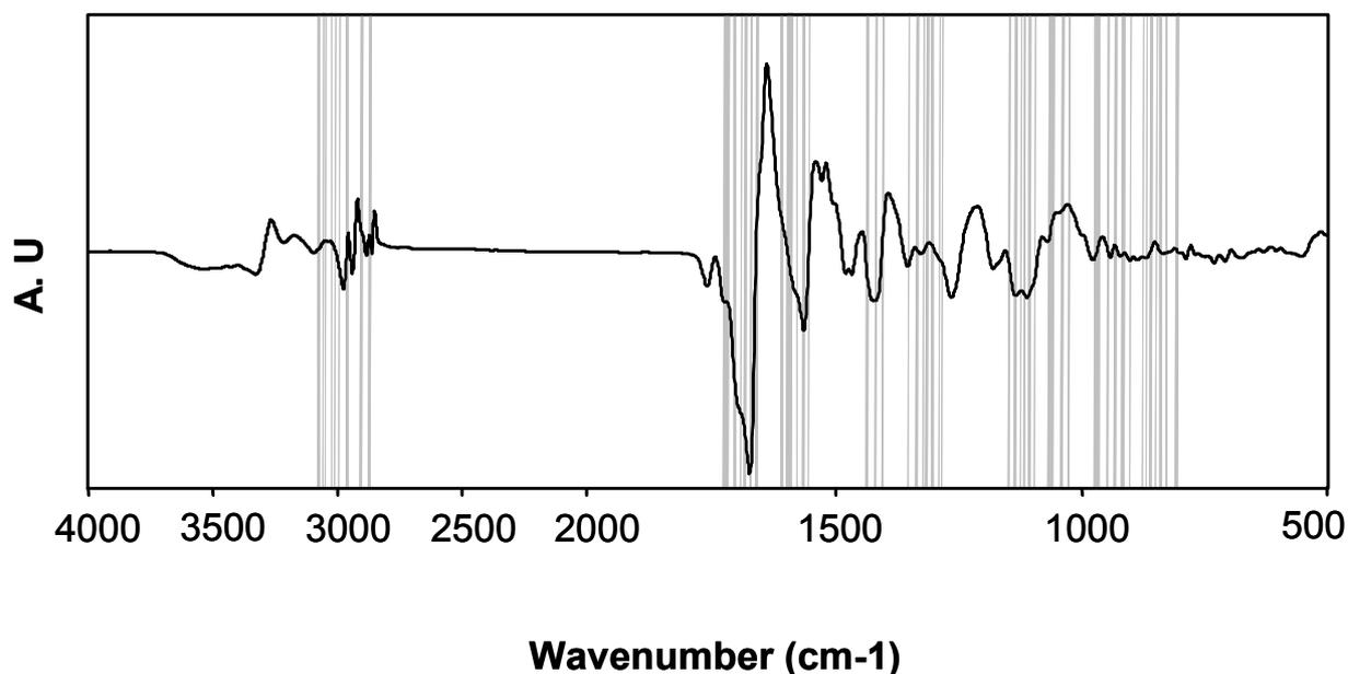
**Fig. 3.1** First derivative of a *Listeria* FTIR spectrum. The regions of the infrared spectra contributing most significantly to the differentiation of the five *Listeria* species are highlighted. A.U., arbitrary units.
