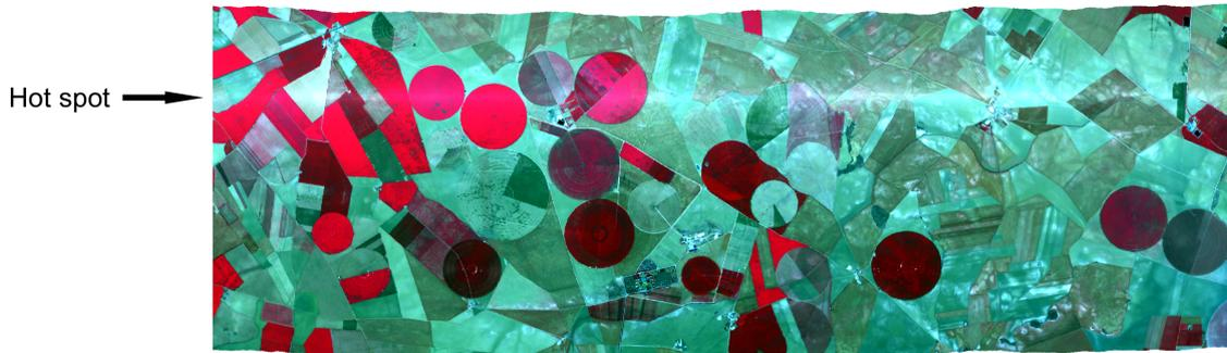
Figure 2.9: Hot spot effect in HyMap airborne imagery. False color image of Barrax, Spain (acquired on June 3, 1999 at solar noon)
