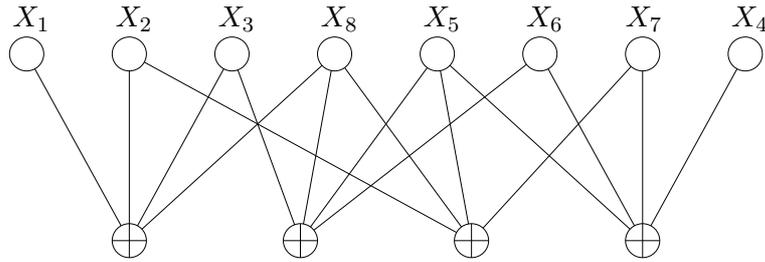
**Figure 3.2:** Tanner graph representation of the (8,4,4) extended Hamming code based on  $G_{MSGM}$  with a minimum loop size of four.
