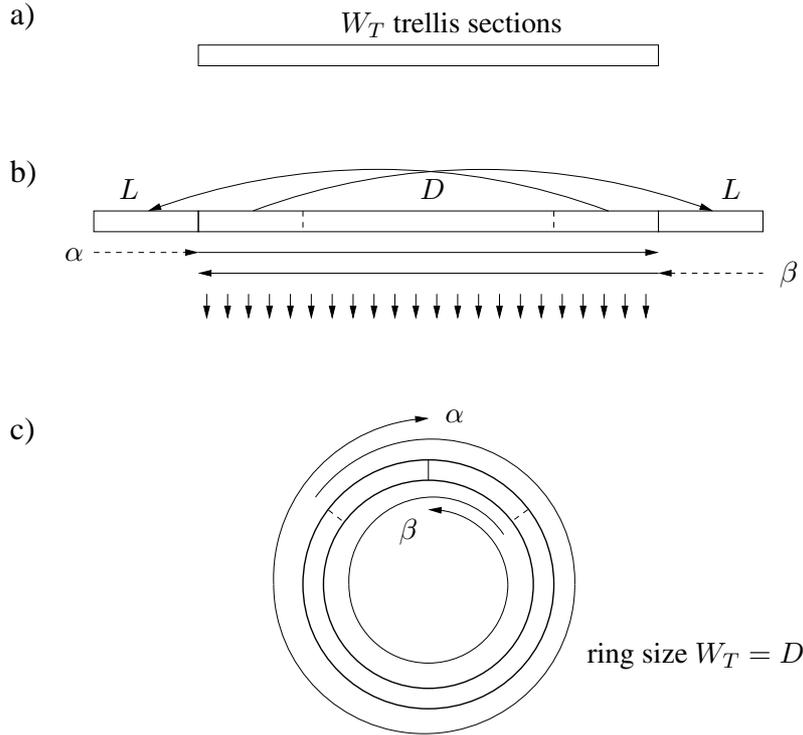
**Figure 4.8:** a) Unwrapped trellis of a tailbiting code. b) Decoding of a tailbiting code as a special case of the generalized sliding window decoding algorithm. c) Decoding of a tailbiting code with the wrap around algorithm.
