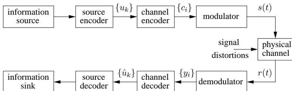
Figure 2.1: Block diagram of a digital communication system.
