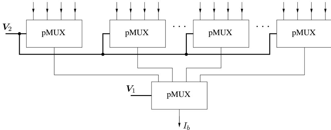
**Figure 6.10:** The stacked configuration of probability multiplexors for probability multiplication.
