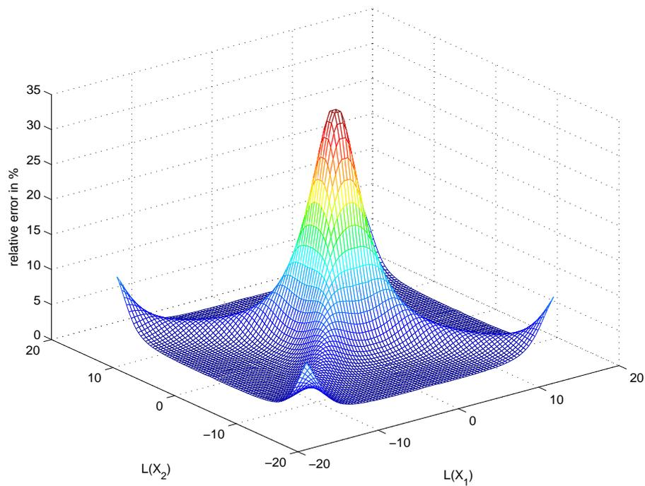
**Figure 8.13:** Relative error of the BPX building block at 27 °C.
