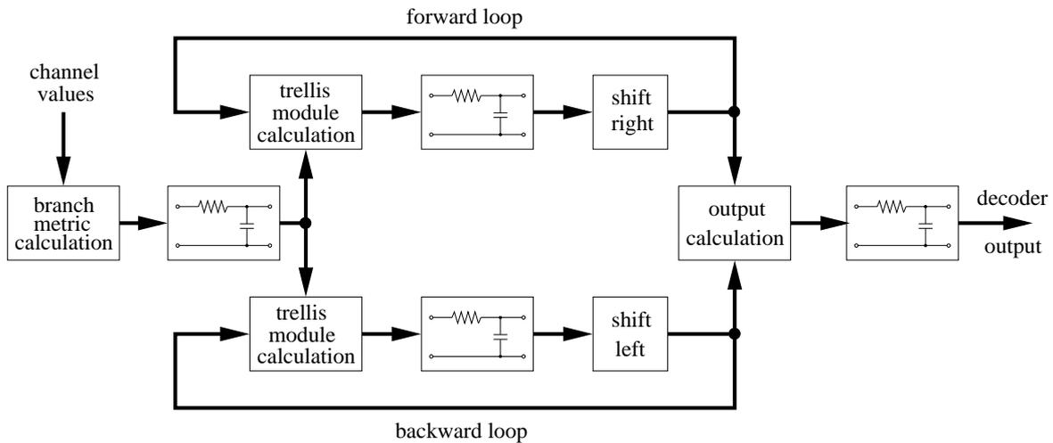
**Figure 5.15:** Time-continuous simulation model of an analog tailbiting convolutional decoder.
