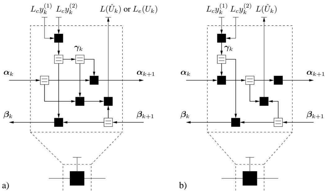
**Figure 5.14:** Implementation of a node processor in a convolutional decoder for codes with systematic feedback encoder in a) and for codes with feedforward encoder in b).
