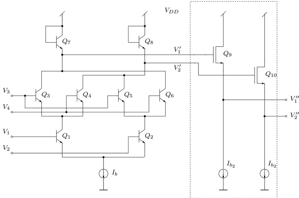
Figure 6.13: The Boxplus circuit with CMOS voltage-shifting output stage.
