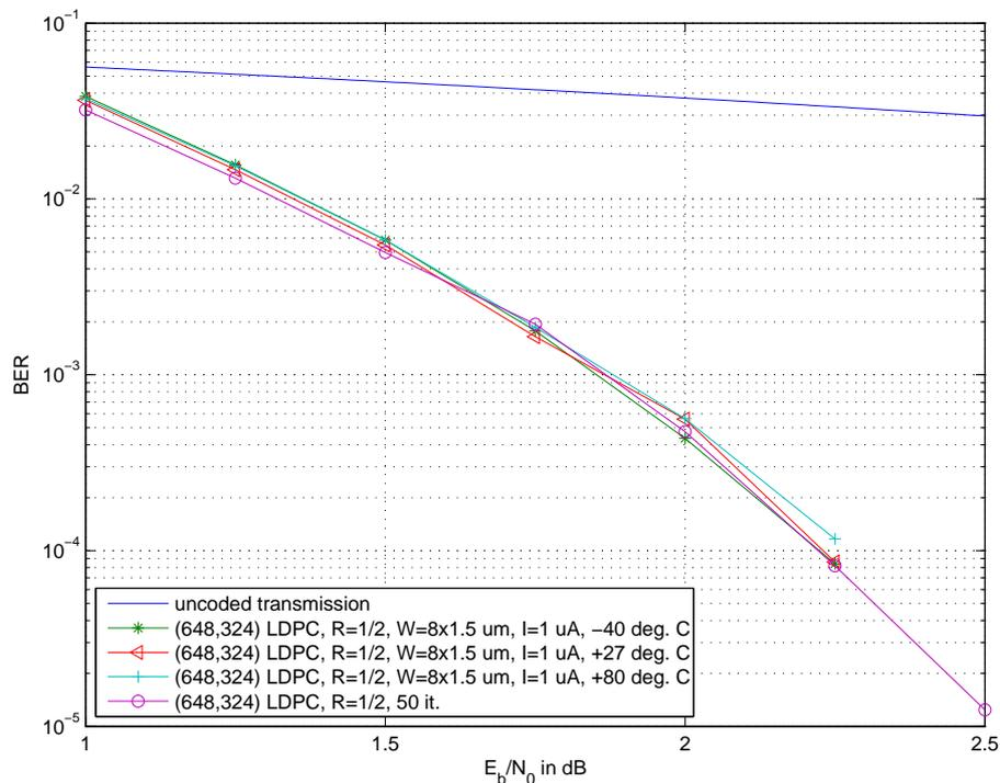
**Figure 8.11:** Estimated BER of the  $R = 1/2$  analog LDPC decoder at different temperatures (with trimming).
