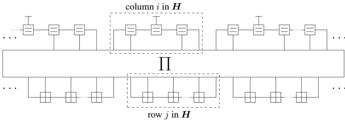
**Figure 3.10:** Transformed normal graph of a generic LDPC code with degree three nodes.
