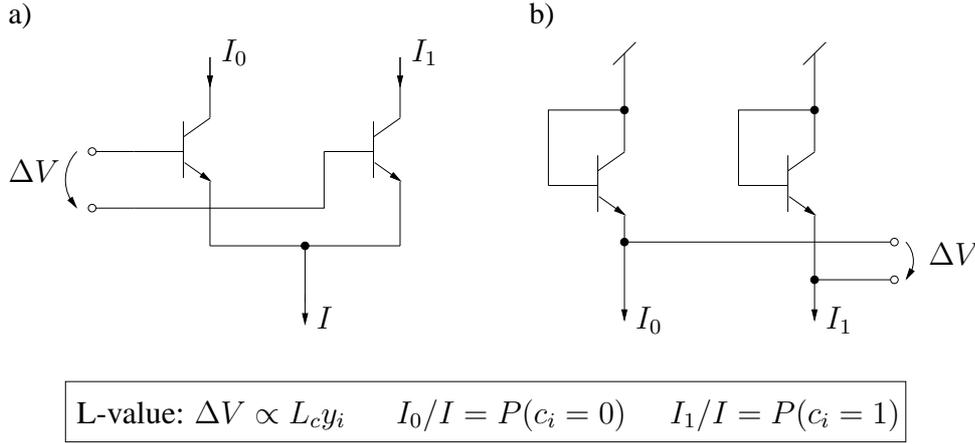
**Figure 2.9:** Conversion of a L-value into the corresponding probabilities in a) and the conversion of the probabilities back to a L-value in b).
