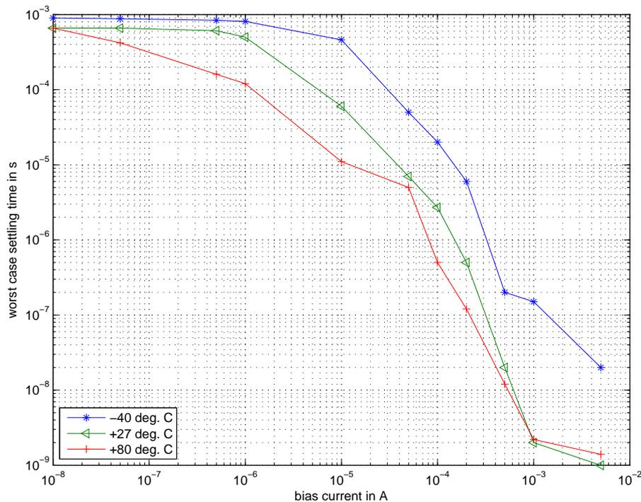
**Figure 8.17:** Worst case settling time of the analog decoding network at different temperatures (settling to 98 % of the largest possible magnitude at the output).
