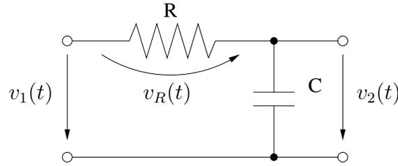
**Figure 5.3:** Basic RC element consisting of a resistor and capacitor.
