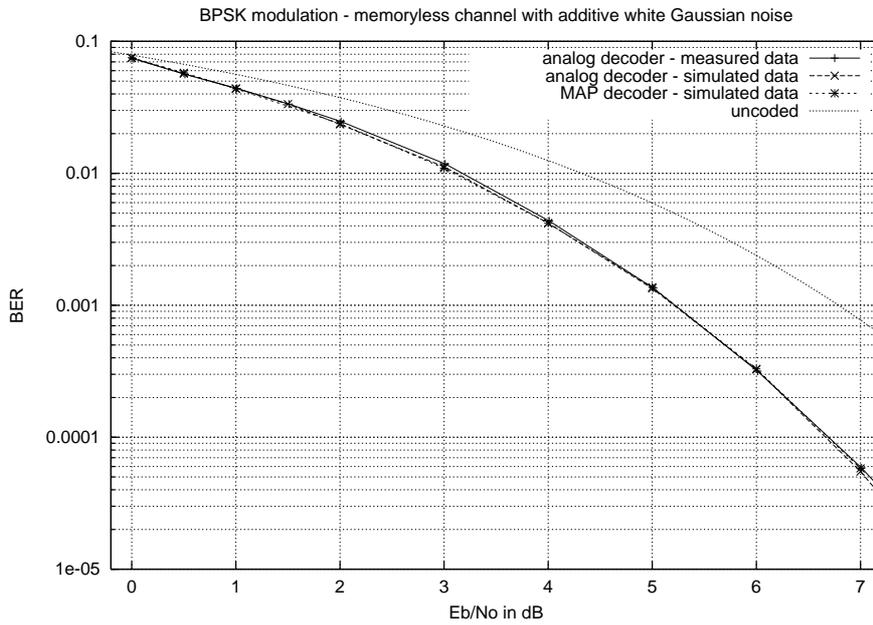
Figure 7.8: Simulated and measured BER of the BiCMOS decoder chip.
