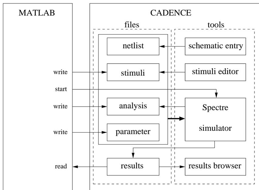
**Figure 5.4:** Link between MATLAB and the CADENCE design environment.
