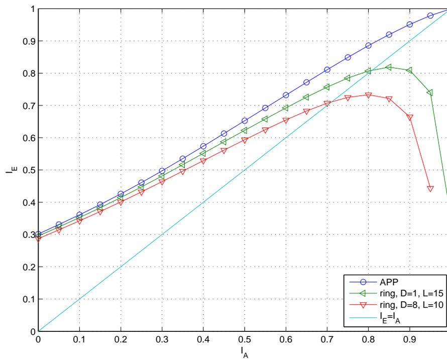
**Figure 5.21:** Characteristic curves of different decoders for the (512,256) tailbiting convolutional code at a  $E_b/N_0$  value of 1 dB.
