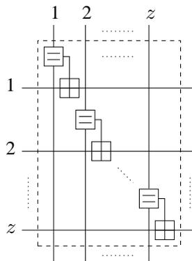
**Figure 8.4:** Block diagram of a layout module in Fig. 8.2 and Fig. 8.3.
