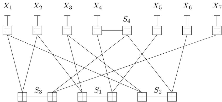
**Figure 5.8:** Decoding network for the (7,4,3) Hamming code based on the  $7 \times 11$  extended  $H$  matrix.
