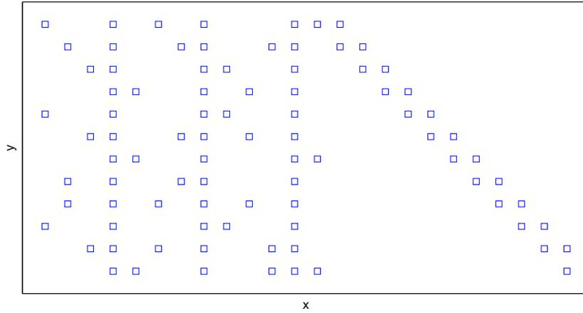
**Figure 8.2:** Top-level layout of the (648,324) LDPC decoder core based on the parity-check matrix (without area optimization).
