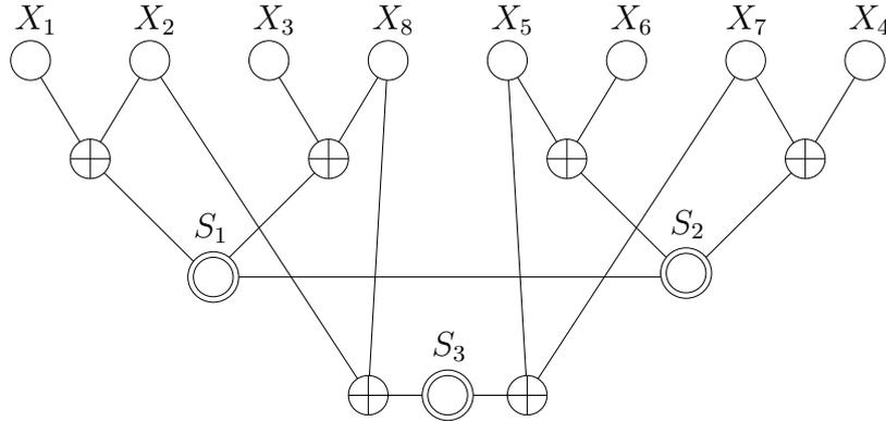
**Figure 3.4:** Factor graph representation of the (8,4,4) extended Hamming code with minimum girth six.
