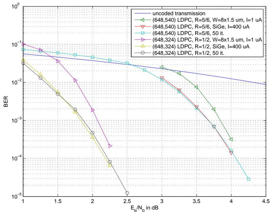
**Figure 8.8:** Estimated BER of the analog LDPC decoders implemented in SiGe and CMOS technology at room temperature (no trimming).
