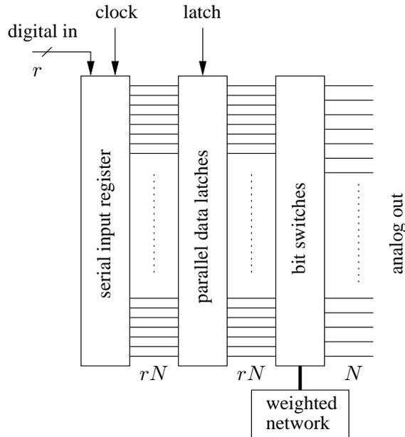
**Figure 8.5:** Digital input interface of the analog LDPC decoder including D/A conversion.
