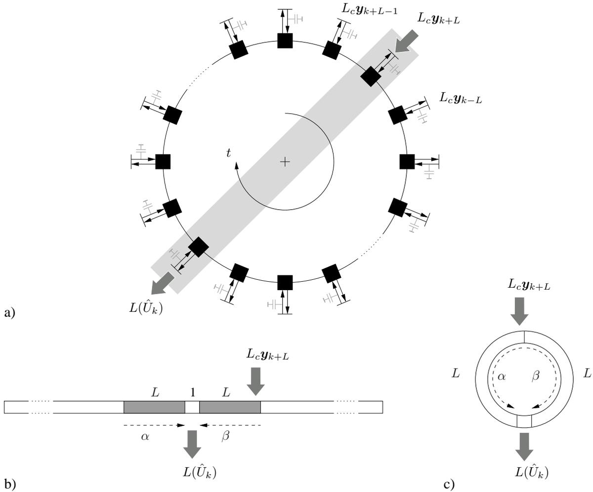
**Figure 5.17:** Basic concept of the ring decoder with  $D = 1$  and  $W = 2L + 1$ .
