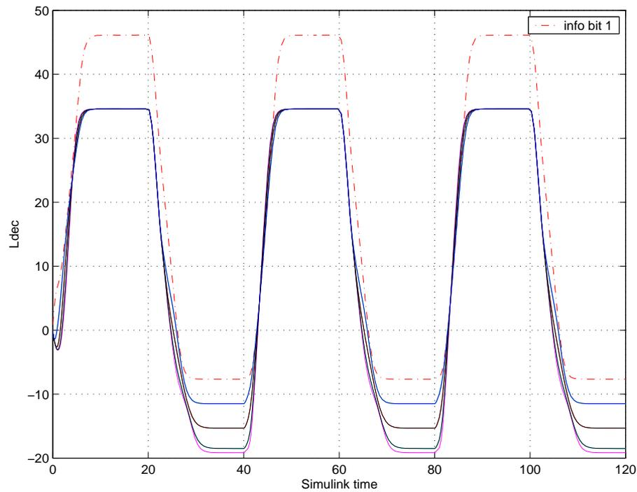
**Figure 7.4:** Transient behavior of the L-values at the output of the ideal analog decoder for the switching input configuration in Fig. 7.3 (transmission error in the first bit position of  $u_b$  is corrected).
