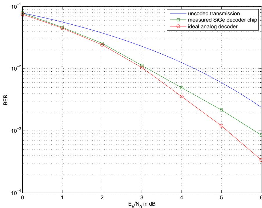
**Figure 7.15:** Simulated and measured BER of the SiGe decoder chip.
