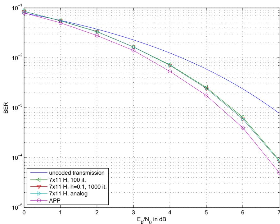
**Figure 5.9:** Decoding of the (7,4,3) Hamming code based on the  $7 \times 11$  extended  $H$  matrix.
