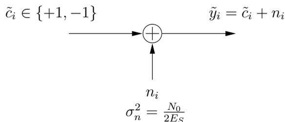
**Figure 2.4:** Normalized AWGN channel model.
