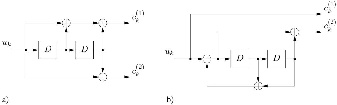
**Figure 2.7:** Encoder realizations for a rate  $R = 1/2$  and memory  $m = 2$  convolutional code (feedforward encoder in a) and recursive systematic encoder in b) ).
