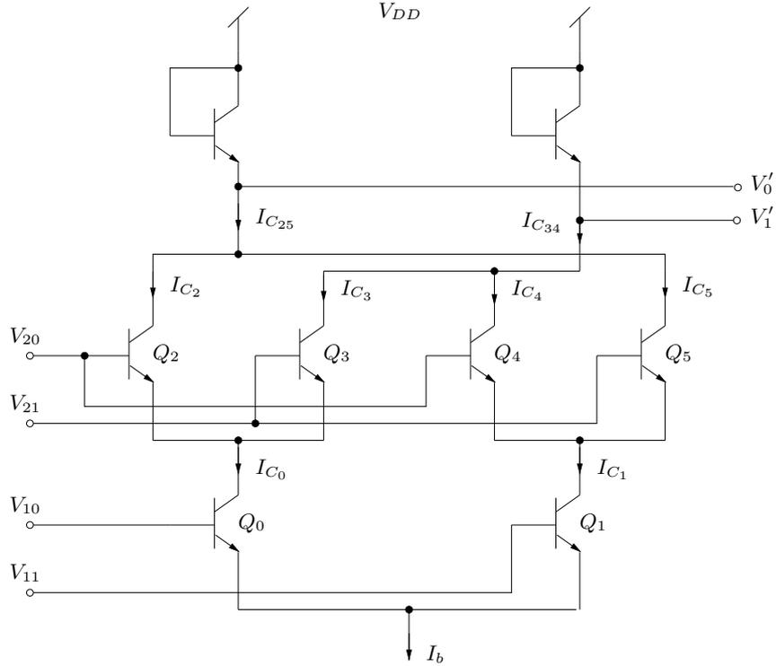
**Figure 6.6:** The Boxplus circuit consisting of a Gilbert multiplier and a pair of diode-connected transistors stacked on top.
