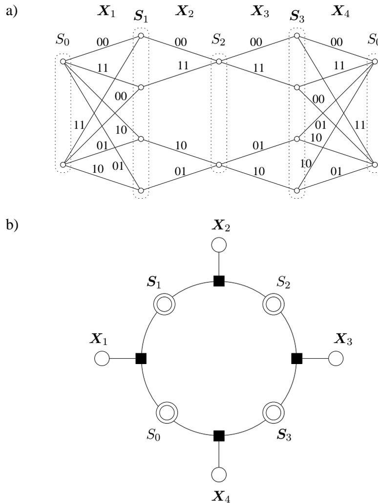
**Figure 3.6:** Minimal tailbiting trellis representation of the  $(8,4,4)$  extended Hamming code with a state space dimension profile of  $(2,4,2,4,2)$  in a) and the associated factor graph in b).
