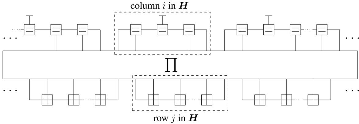
**Figure 5.34:** Generic view of an analog LDPC decoder.
