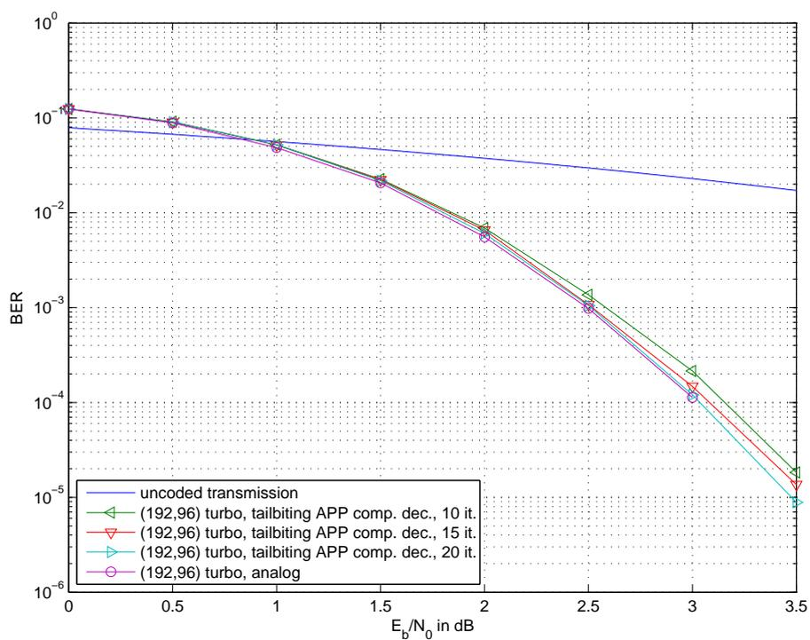
**Figure 5.29:** Decoding of the (192,96) DVB turbo code with memory three tailbiting convolutional codes as component codes.
