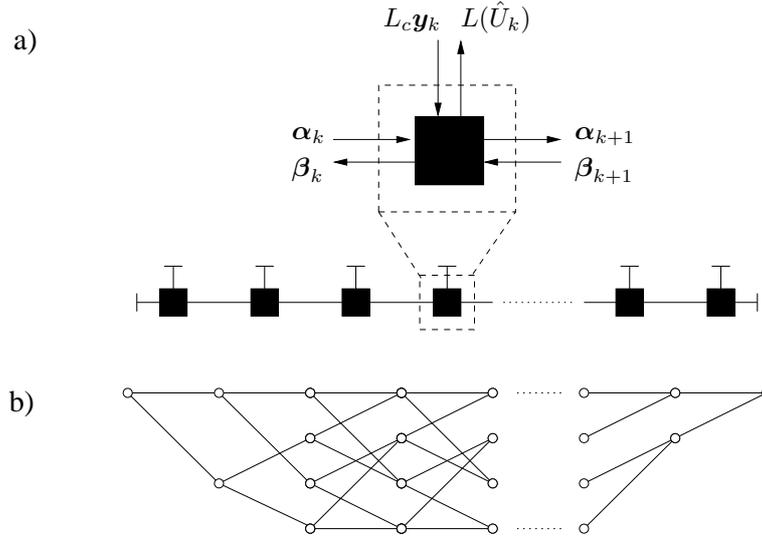
**Figure 4.5:** Normal graph of a terminated convolutional code with an exposed message flow for generalized constraint node  $k$  in a) and the equivalent trellis representation for the example of a memory  $m = 2$  code in b).
