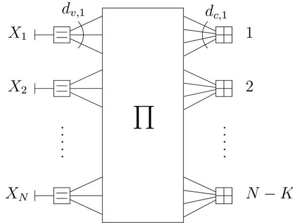
**Figure 3.9:** Normal graph representation of a generic LDPC code.
