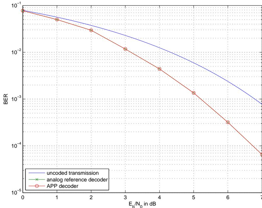
**Figure 7.1:** Simulated BER for the (16,8,3) tailbiting convolutional code.
