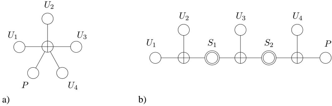
**Figure 3.3:** Two different factor graph representations of the (5,4,2) SPC code.
