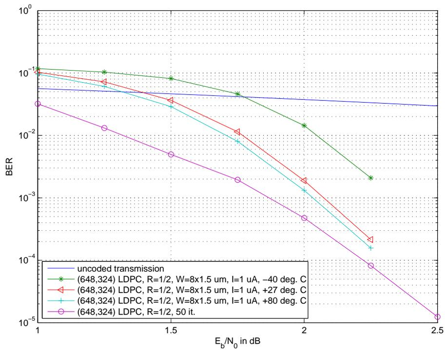
**Figure 8.9:** Estimated BER of the  $R = 1/2$  analog LDPC decoder at different temperatures (no trimming).
