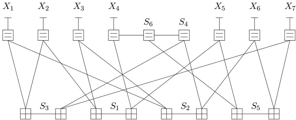
**Figure 5.10:** Decoding network for the (7,4,3) Hamming code based on the  $10 \times 13$  extended  $H$  matrix with a redundant parity-check.
