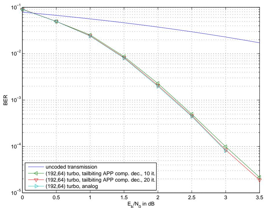
**Figure 5.28:** Decoding of the (192,64) turbo code with memory two tailbiting codes as component codes.
