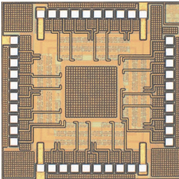
**Figure 7.19:** Die micrograph of our SiGe decoder implementation.
