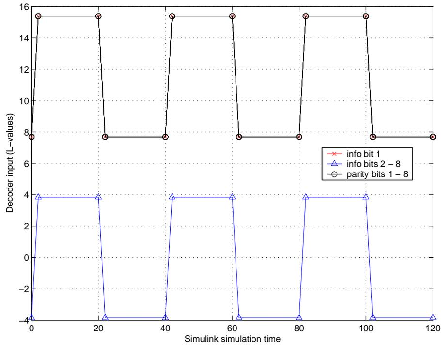
**Figure 7.3:** Switching between the channel values for code word  $c_a$  and  $c_b$  with a transmission error in the first bit position of  $c_b$ .
