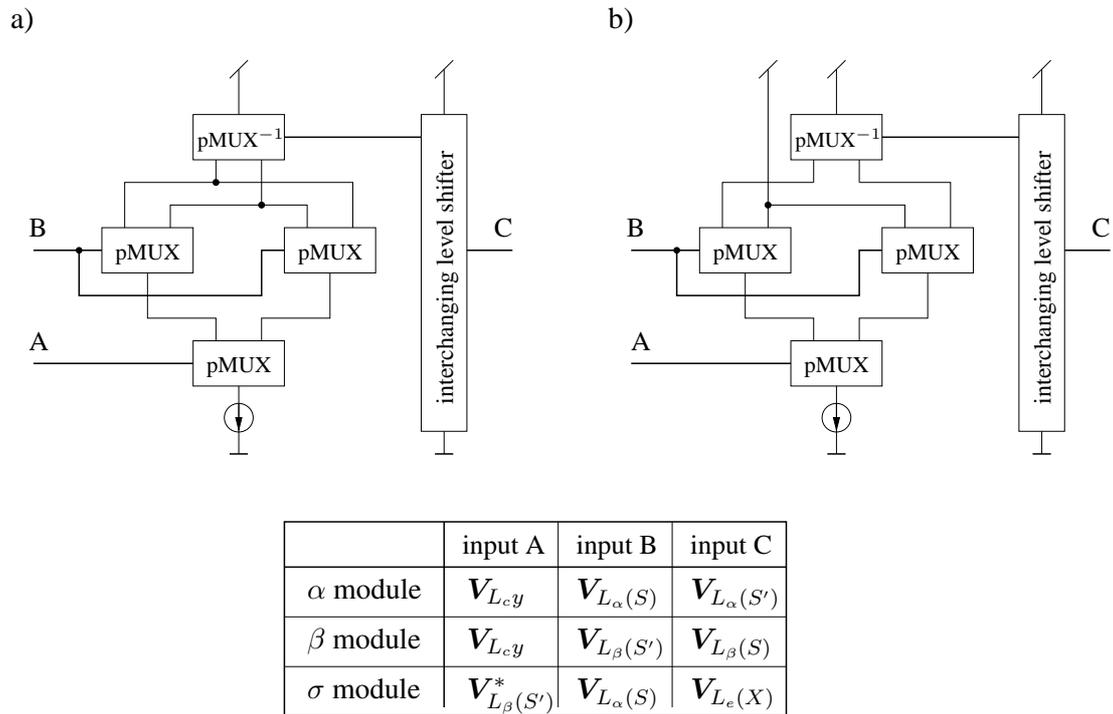
**Figure 6.17:** Schematic of the  $\alpha$ ,  $\beta$  and  $\sigma$  modules in a check node processor in a) and an equality node processor in b).
