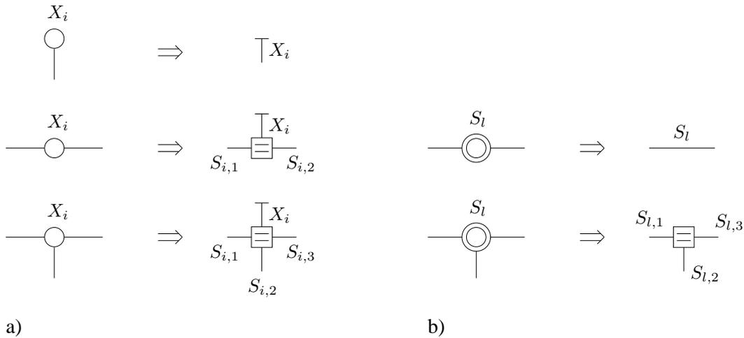
**Figure 3.7:** Conversion of symbol and state variable nodes in factor graphs into the corresponding normal graph representation.
