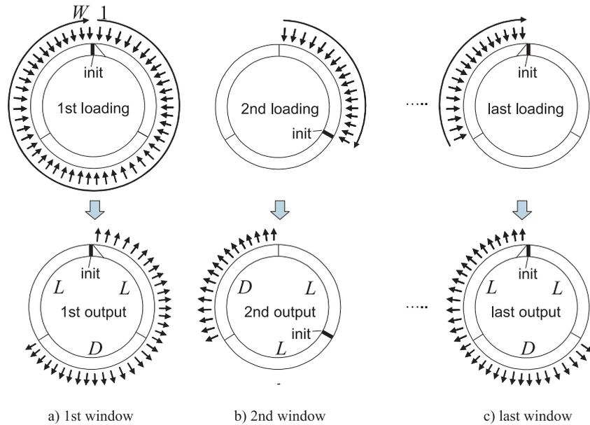
**Figure 5.22:** Loading and unloading of the SwinDec decoder with  $D = L = W/3$  for the case of a terminated convolutional code.
