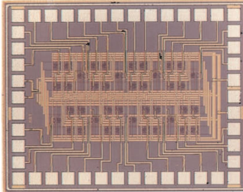
**Figure 7.18:** Die micrograph of our BiCMOS decoder implementation.
