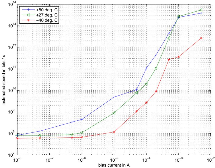
Figure 8.19: Estimated speed of the (648,540) analog LDPC decoder at different temperatures.
