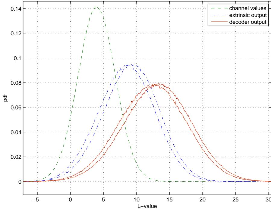
**Figure 5.19:** Comparison between the distributions of absolute L-values of the ring decoder with  $D = 8$ ,  $L = 10$  and the APP decoder at a  $E_b/N_0$  value of 3 dB.
