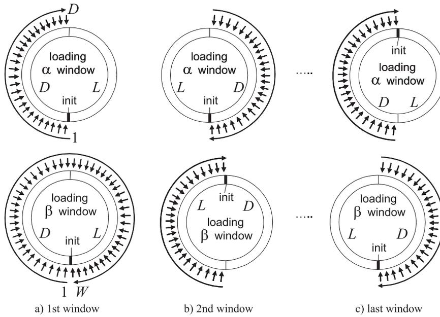
**Figure 5.24:** Loading of the modified SwinDec decoder with  $D = L = W'/2$  for the case of a terminated convolutional code.
