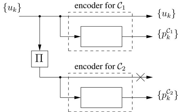
**Figure 2.8:** Encoder for the parallel concatenation of two rate  $R = 1/2$  convolutional codes with recursive systematic encoder.
