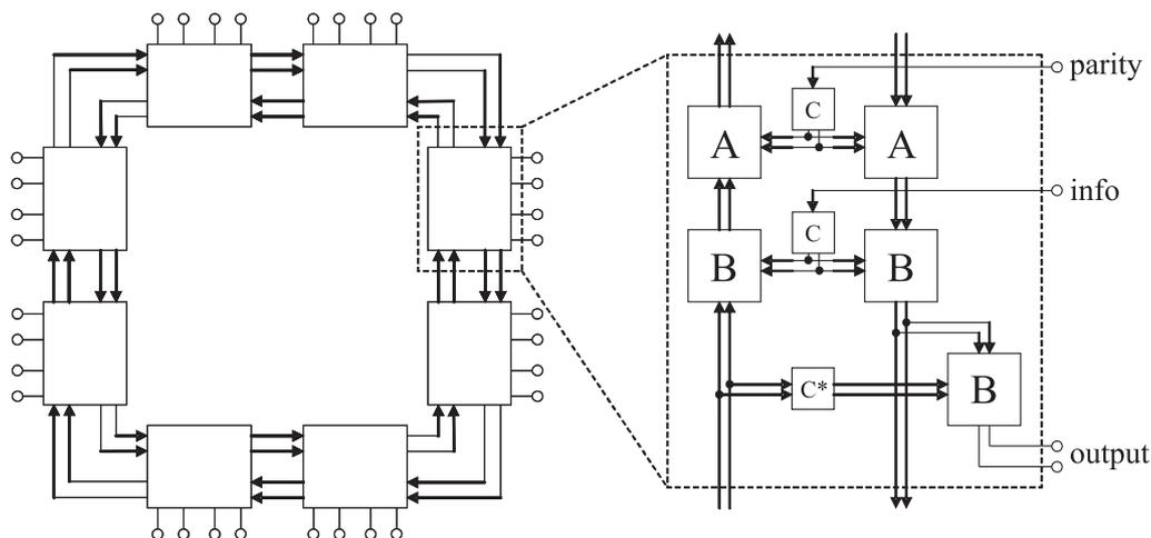
Figure 7.11: Block diagram of the SiGe decoder chip.
