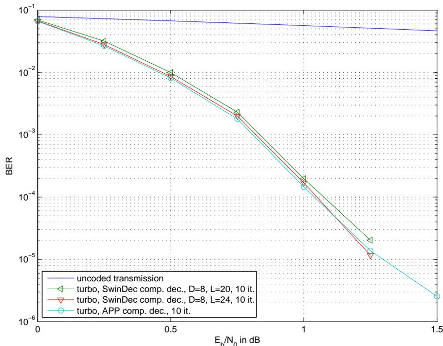
**Figure 5.31:** Decoding of the (1932,640) UMTS turbo code with different SwinDec component decoder configurations.
