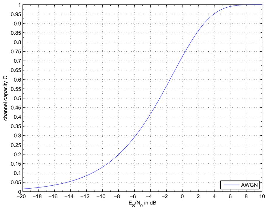
**Figure 2.10:** Channel capacity of the binary input AWGN channel over  $E_S/N_0$ .
