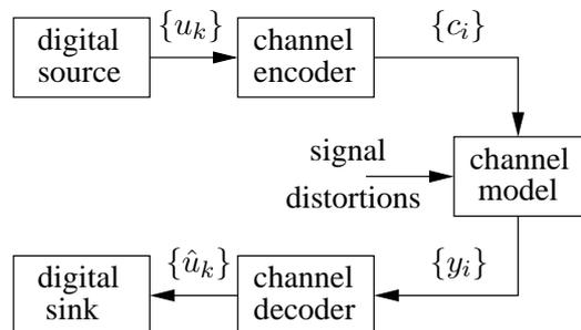
**Figure 2.2:** Simplified model of a digital communication system.
