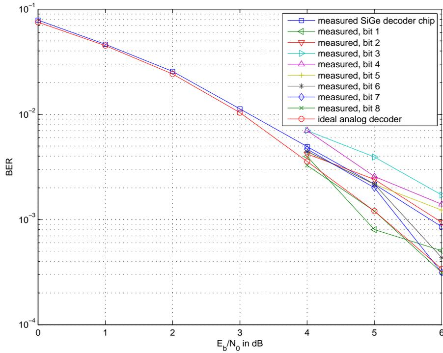
**Figure 7.16:** Measured BER of the SiGe decoder chip together with the measured BER for the individual bit positions.
