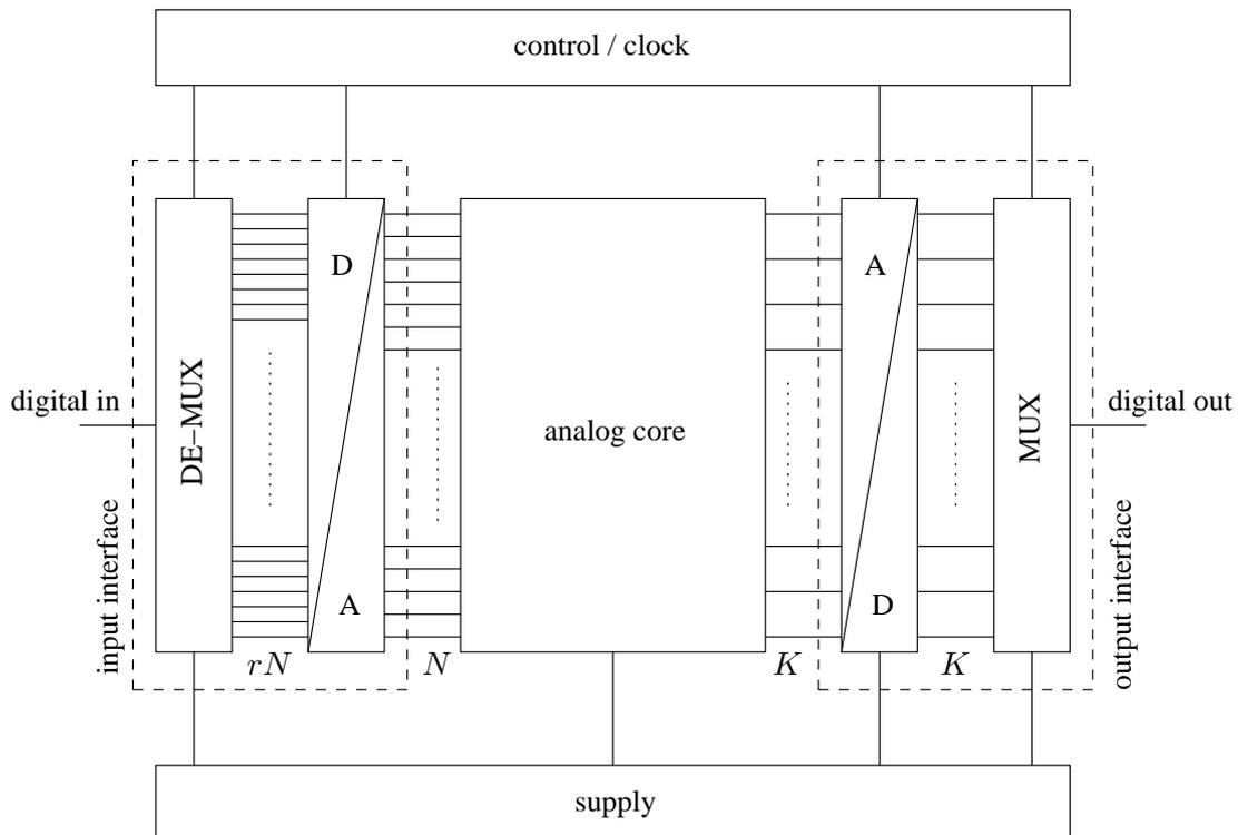
**Figure 8.1:** Block diagram of the analog LDPC decoder with digital input and output interfaces.
