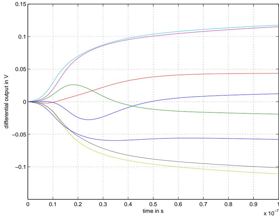
**Figure 7.7:** Circuit simulation of the BiCMOS decoder chip at 0° C (reference decoding situation).
