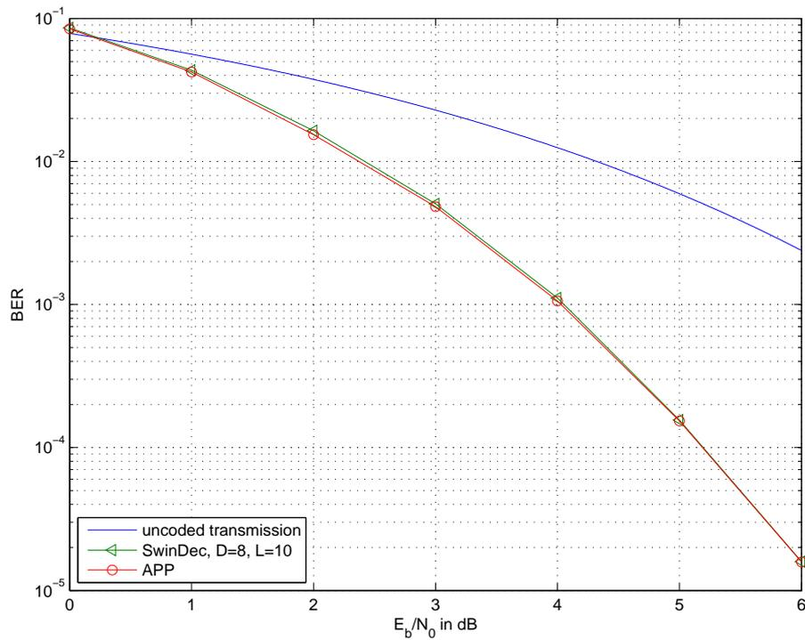
**Figure 5.26:** Decoding of the (512,256) tailbiting convolutional code with the SwinDec decoder.
