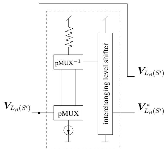
**Figure 6.18:** Schematic of the equality module in the SPC decoder (voltage level shifter).
