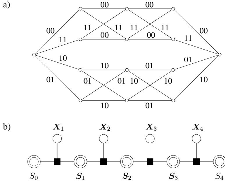
**Figure 3.5:** Minimal trellis representation of the (8,4,4) extended Hamming code with a state space dimension profile of (1,4,4,4,1) in a) and the associated factor graph in b).
