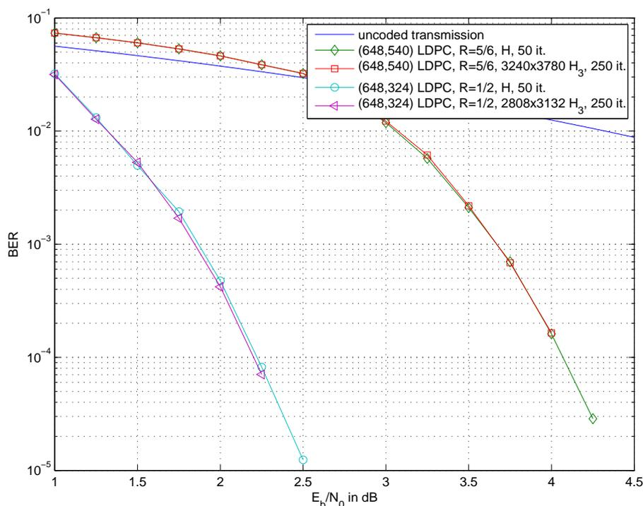
**Figure 5.36:** Decoding of the (648,324) LDPC code with rate  $R = 1/2$  and the (648,540) LDPC code with rate  $R = 5/6$  based on the corresponding  $\mathbf{H}$  and  $\mathbf{H}_3$  matrices.
