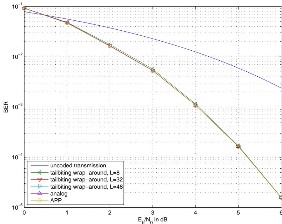
Figure 5.16: Decoding of the (32,16) tailbiting code with memory two.
