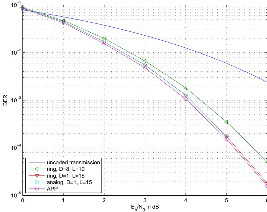
**Figure 5.18:** Decoding of the (512,256) tailbiting convolutional code with different configurations of the ring decoder.
