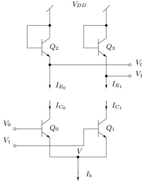
**Figure 6.4:** Differential pair (bottom) and pair of diode-connected transistors (top).
