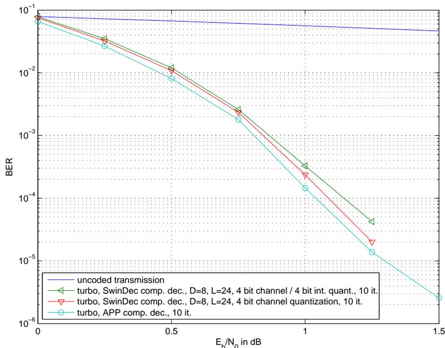
**Figure 5.33:** Decoding of the (1932,640) UMTS turbo code with different component decoders and 4 bit quantization.
