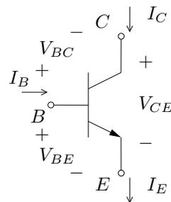
**Figure 6.1:** A bipolar npn transistor with sign convention.
