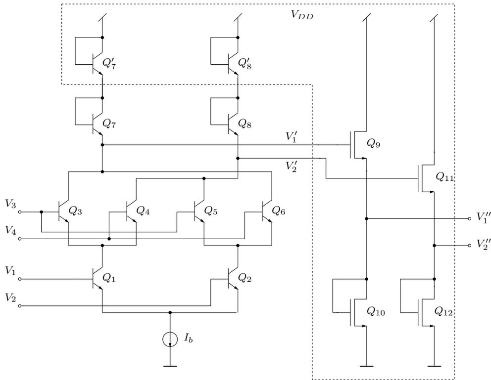
**Figure 6.12:** The (modified) Boxplus circuit with CMOS voltage-dividing output stage.
