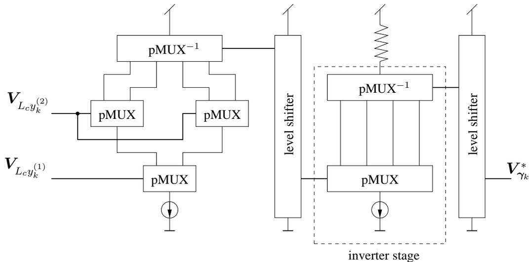
**Figure 6.20:** Schematic of the  $\gamma$  module in the convolutional decoder.
