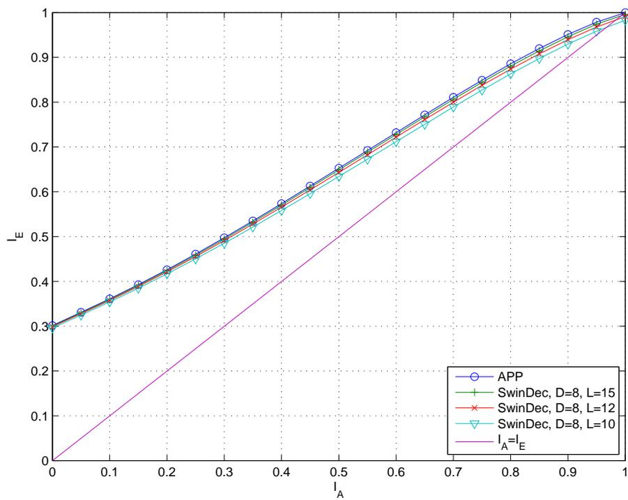
**Figure 5.27:** Characteristic curves of different SwinDec decoder configurations for the (512,256) tailbiting convolutional code at a  $E_b/N_0$  value of 1 dB.
