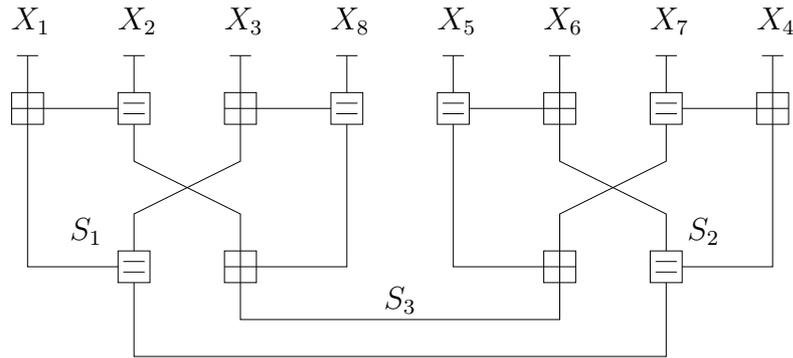
**Figure 3.8:** Normal graph representation of the (8,4,4) extended Hamming code with minimum girth six.
