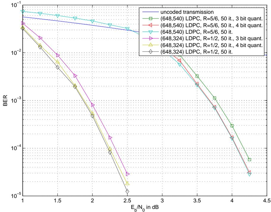
**Figure 5.37:** Decoding of the (648,324) LDPC code with rate  $R = 1/2$  and the (648,540) LDPC code with rate  $R = 5/6$  based on the  $\mathbf{H}$  matrices with a quantization of the decoder input.
