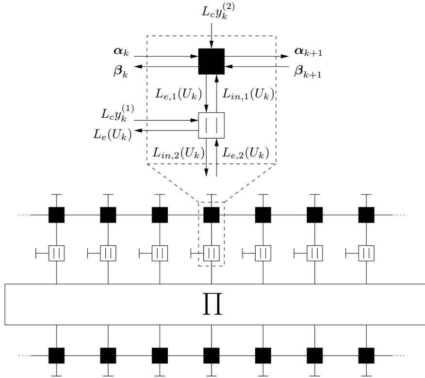
**Figure 4.9:** Normal graph of a turbo code which consists of a parallel concatenation of two rate  $R = 1/2$  convolutional codes.
