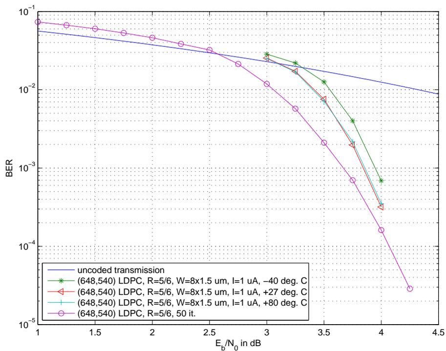
**Figure 8.10:** Estimated BER of the  $R = 5/6$  analog LDPC decoder at different temperatures (no trimming).
