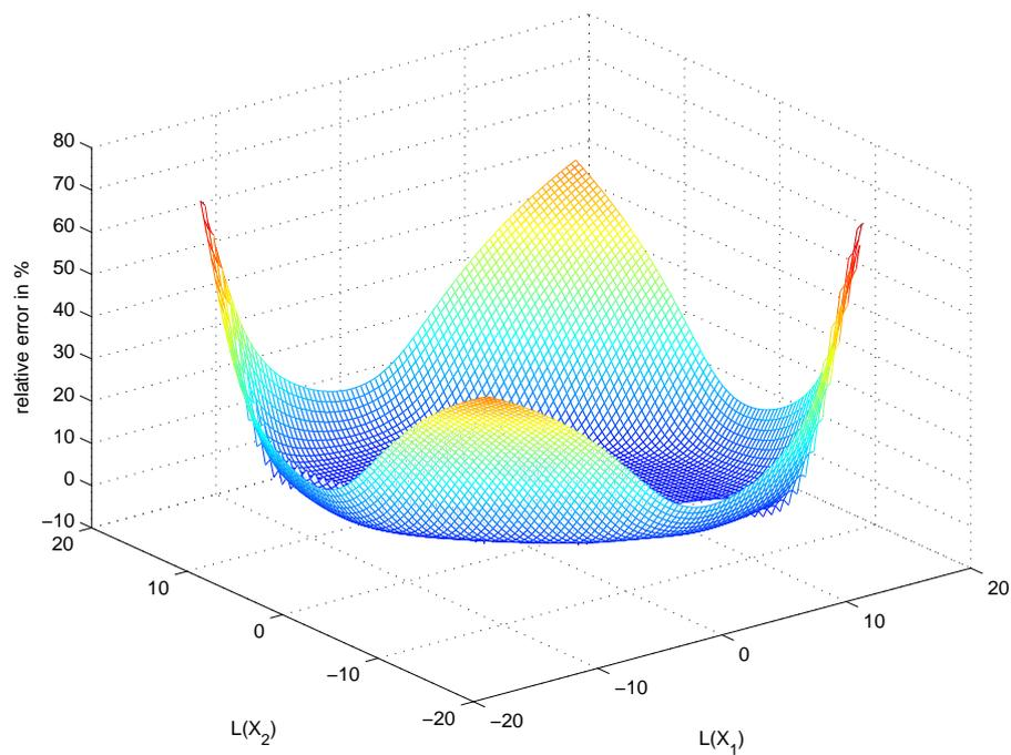
**Figure 8.14:** Relative error of the SUM building block at 27 °C.
