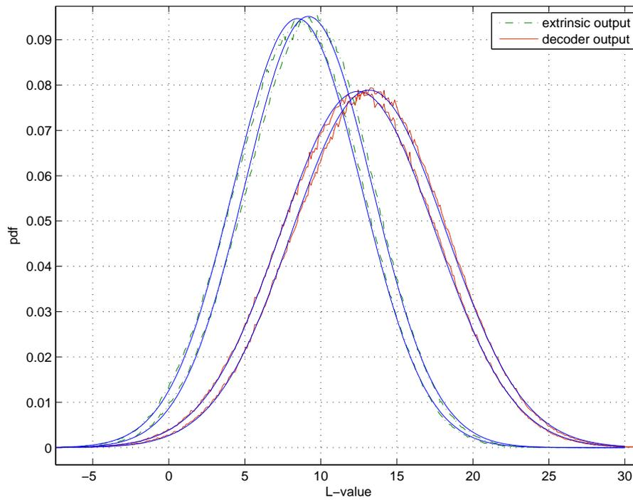
**Figure 5.20:** Comparison between the distributions in Fig. 5.19 and Gaussian distributions according to Table 5.1.
