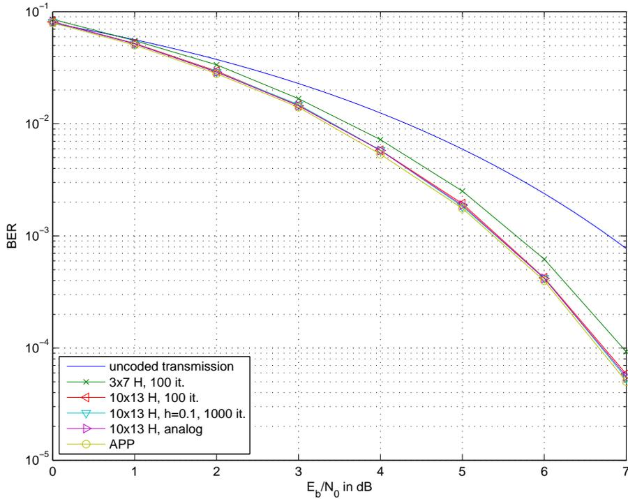
**Figure 5.11:** Decoding of the (7,4,3) Hamming code based on the  $10 \times 13$  extended  $H$  matrix with a redundant parity-check.
