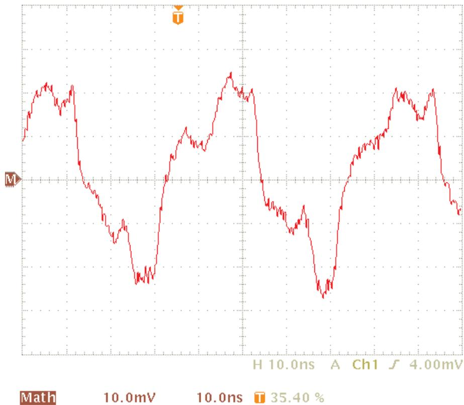
**Figure 7.17:** Transient response of the decoder output for  $u_1$  for the switching between code words  $c_a$  and  $c_b$  with a transmission error in  $u_1$ .
