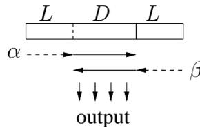
**Figure 4.6:** Generalized sliding window decoder with a window size of  $W = D + 2L$ .
