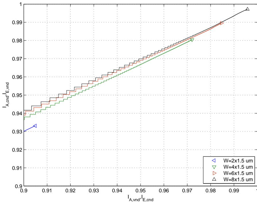
**Figure 8.7:** Trajectories for the  $R = 1/2$  decoder with different transistor widths,  $I_b = 1 \mu\text{A}$  and a  $E_b/N_0$  value of 1.75 dB.
