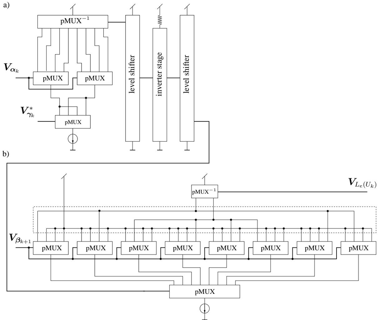
**Figure 6.23:** Schematic of the  $\sigma_1$  module in a) and the  $\sigma_2$  module in b) for the calculation of the extrinsic output in a convolutional decoder (systematic feedback encoder).
