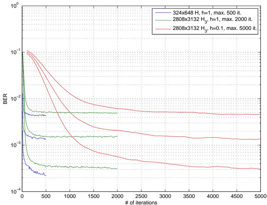
**Figure 5.35:** Simulated BER of different LDPC decoder simulation models for the (648,324) LDPC code at  $E_b/N_0$  values of 1.5 dB, 1.75 dB and 2 dB.
