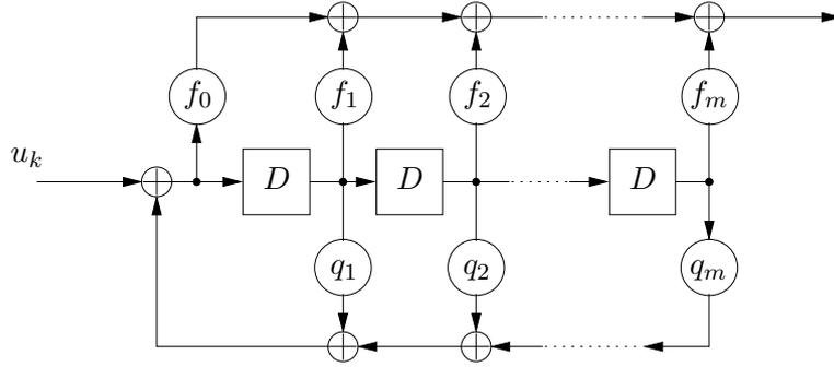
**Figure 2.6:** Realization of the rational transfer function  $g(D)$  in controller canonical form.
