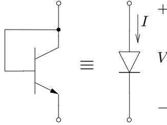
**Figure 6.2:** The diode-connected npn transistor.
