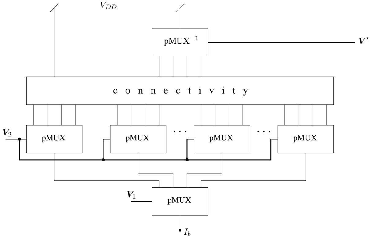
**Figure 6.11:** Structure of the general decoder building block.
