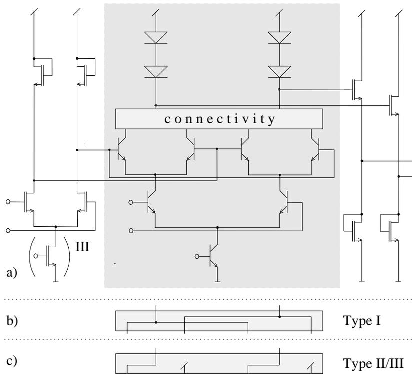
**Figure 7.5:** a) Decoder building block, b) Connectivity for Type I block, c) Connectivity for Type II/III block (III without lower nMOS current source).
