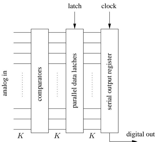
**Figure 8.6:** Digital output interface of the analog LDPC decoder including A/D conversion.
