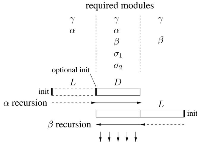
**Figure 6.25:** Required modules for the different sections of the SwinDec decoder.
