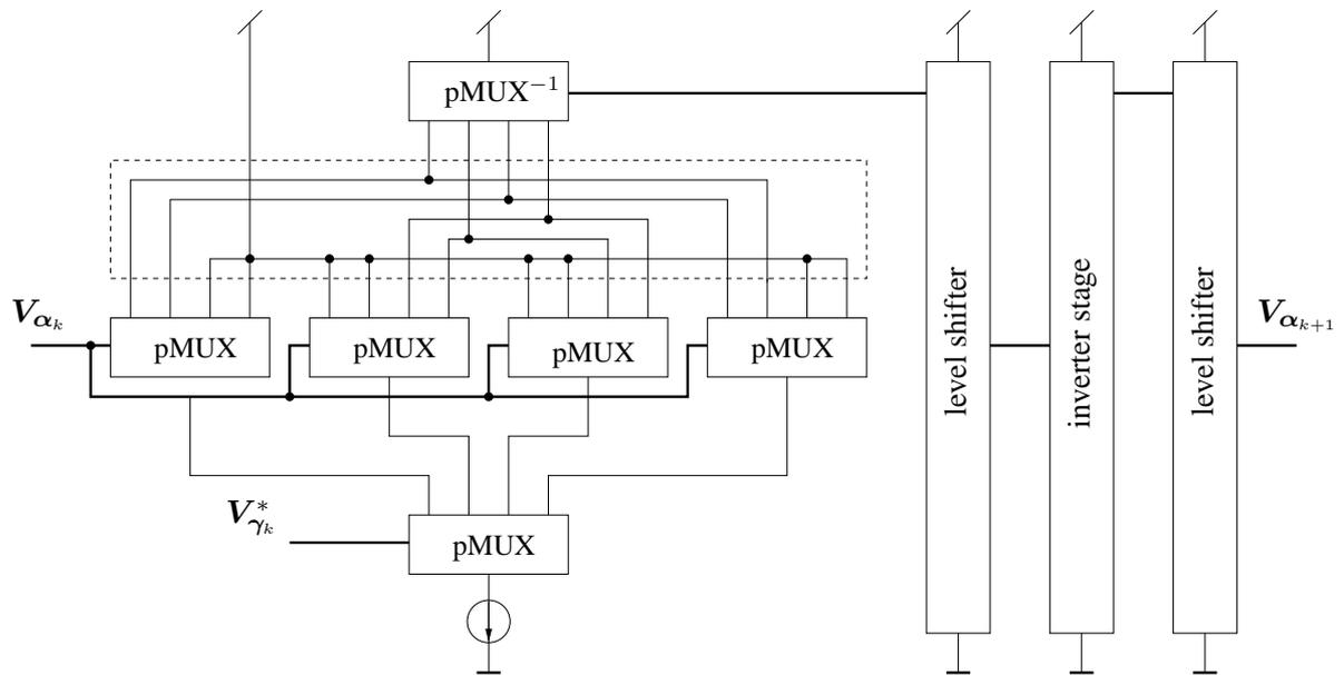
Figure 6.21: Schematic of the  $\alpha$  module in the convolutional decoder.
