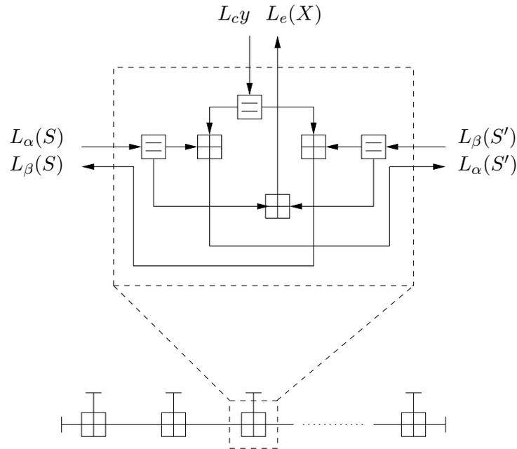
**Figure 5.5:** General check node decoder with a directed view of one check node processor.
