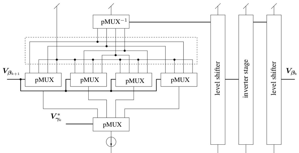
Figure 6.22: Schematic of the  $\beta$  module in the convolutional decoder.
