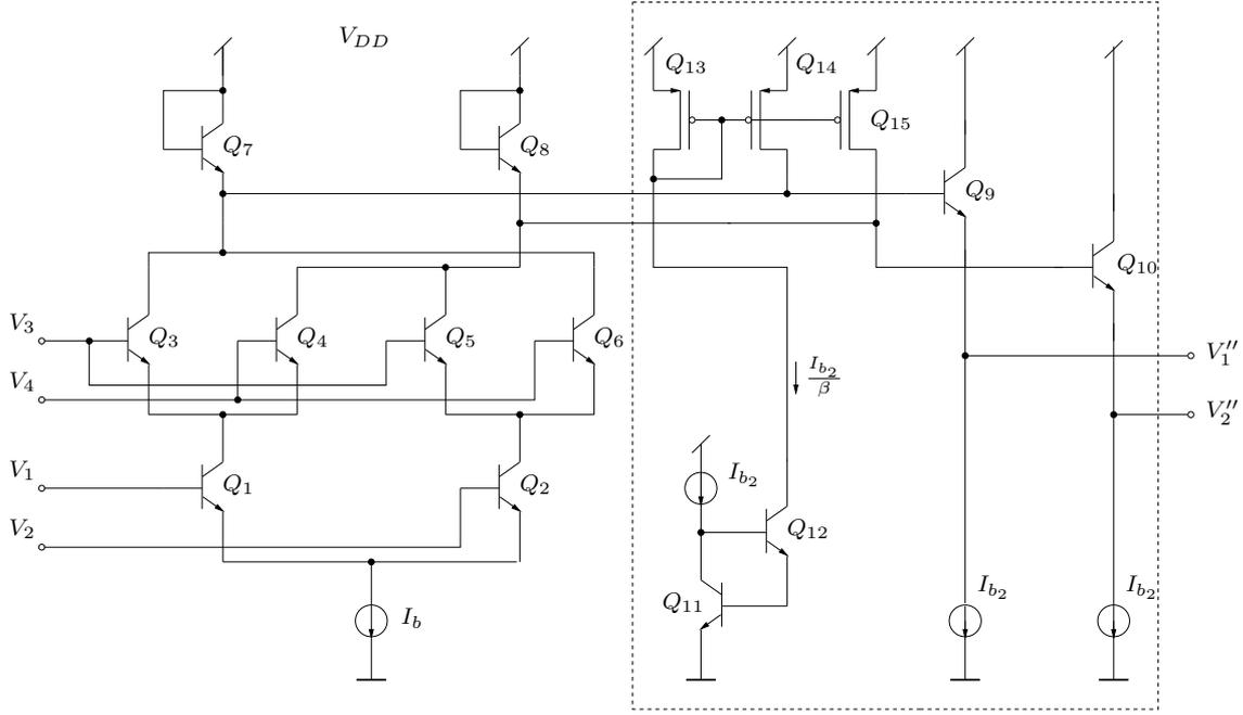
**Figure 6.15:** The Boxplus circuit with bipolar voltage-shifting output stage including load current compensation.
