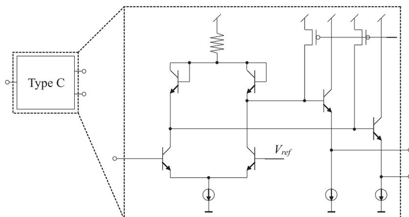
Figure 7.12: Type C decoder building block.
