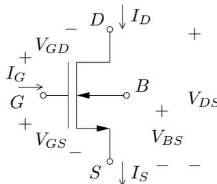
**Figure 6.3:** nMOS transistor with sign convention.
