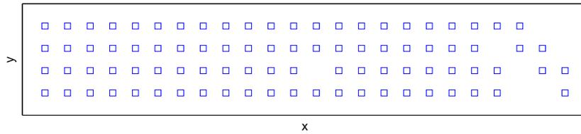
**Figure 8.3:** Top-level layout of the (648,540) LDPC decoder core based on the parity-check matrix (without area optimization).
