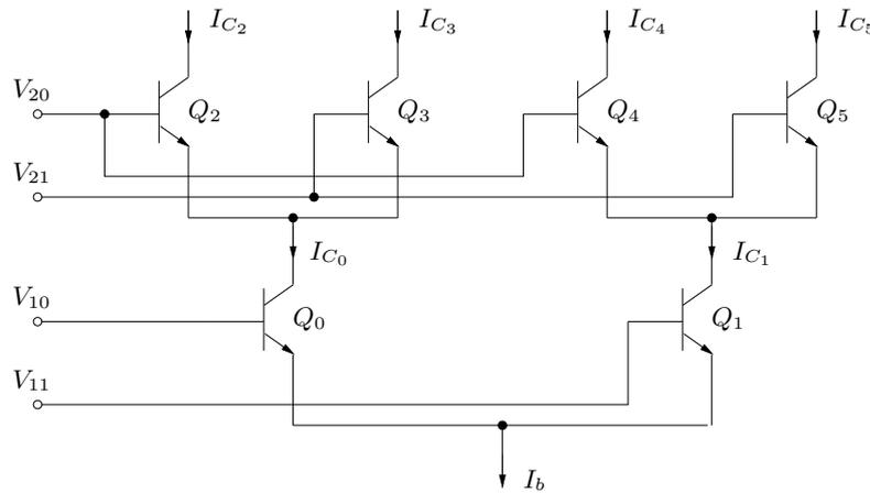
**Figure 6.5:** Stacked configuration of differential pairs.
