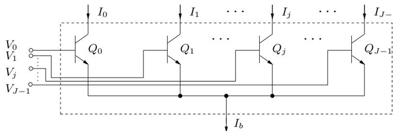
**Figure 6.8:** Probability multiplexor (pMUX) consisting of emitter coupled transistors.
