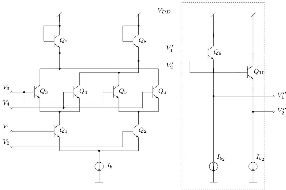
**Figure 6.14:** The Boxplus circuit with bipolar voltage-shifting output stage.
