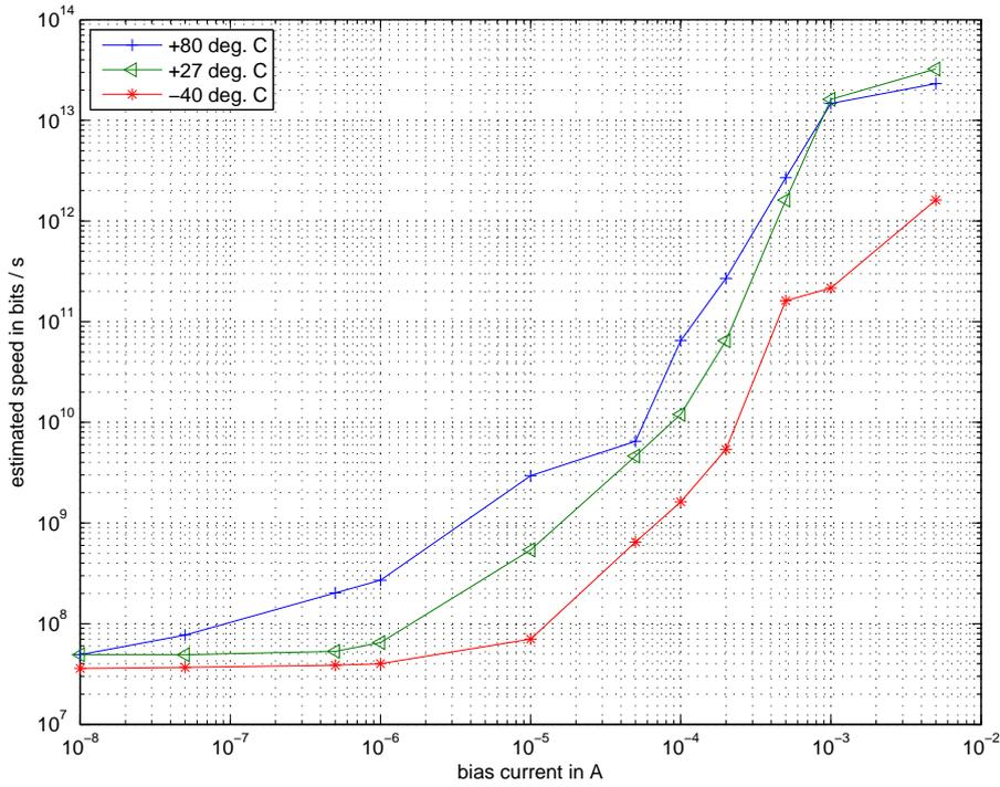
Figure 8.18: Estimated speed of the (648,324) analog LDPC decoder at different temperatures.
