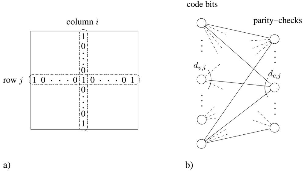
**Figure 2.5:** Example of a row and a column in the parity-check matrix of a LDPC code with  $d_{c,j} = 3$  and  $d_{v,i} = 3$  in a) and the corresponding graph representation of the code in b).
