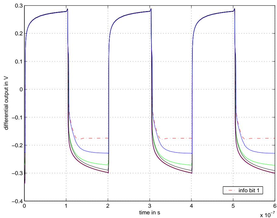
**Figure 7.14:** Circuit-level simulation for the switching input configuration in Fig. 7.3 (transmission error in the first bit position of  $u_b$  is corrected).
