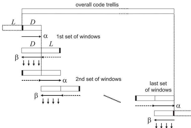
**Figure 5.25:** Unwrapped view of the modified SwinDec decoder in Fig. 5.24 showing the offset between the forward and backward windows.
