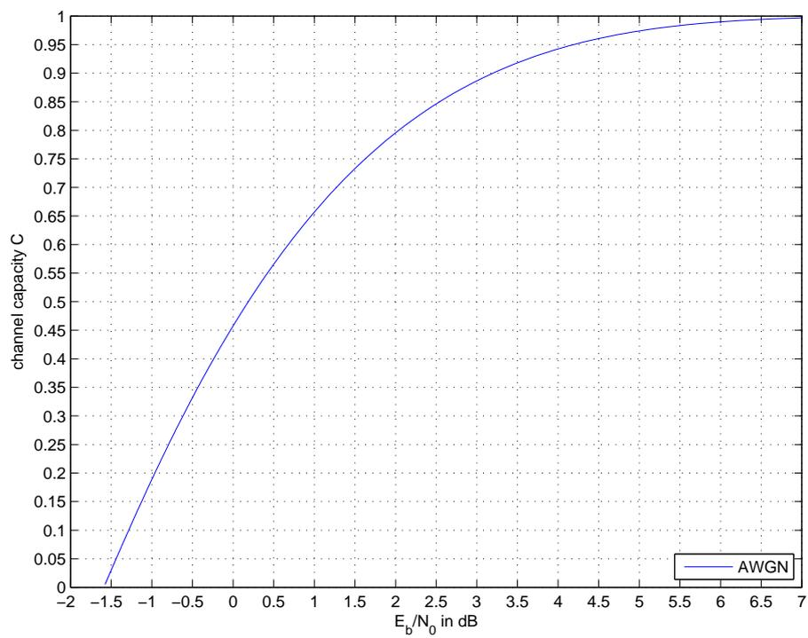
**Figure 2.11:** Channel capacity of the binary input AWGN channel over  $E_b/N_0$ .
