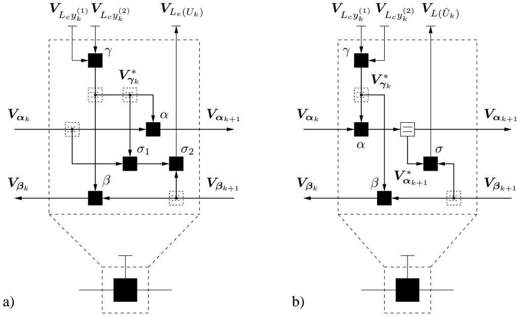
**Figure 6.19:** Block diagram of a node processor for convolutional codes with systematic feedback encoders in a) and feedforward encoders in b).
