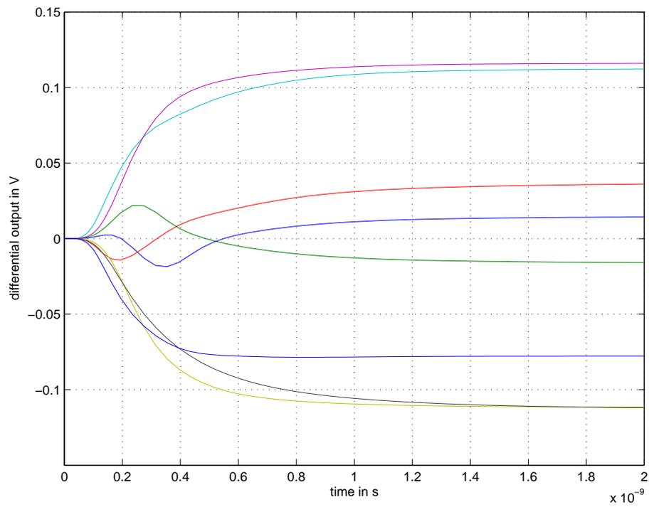
**Figure 7.13:** Circuit-level simulation of the SiGe decoder chip at 25°C (reference decoding situation).
