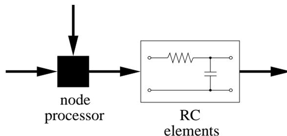
**Figure 5.2:** Time-continuous simulation model for a directed node in the code graph.
