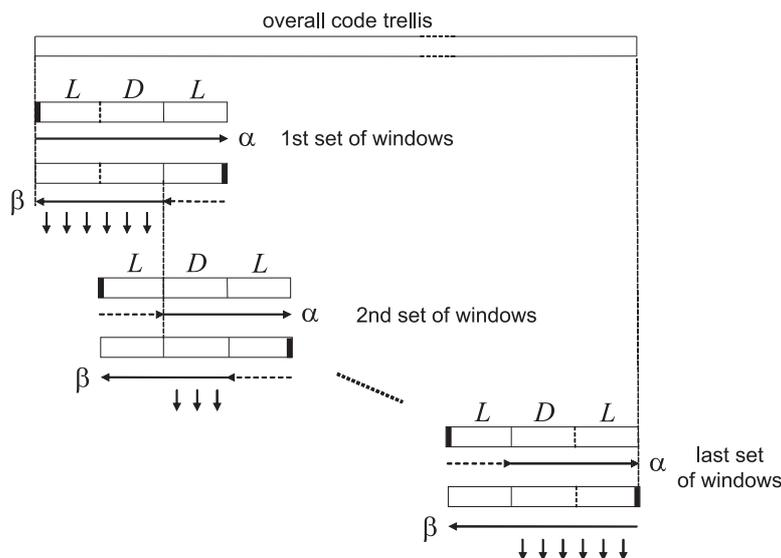
**Figure 5.23:** Unwrapped view of the SwinDec decoder in Fig. 5.22 showing the forward and backward recursions.
