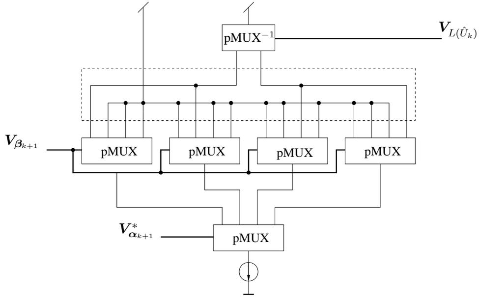
**Figure 6.24:** Schematic of the  $\sigma$  module for the calculation of the decoder output in a convolutional decoder (feedforward encoder).
