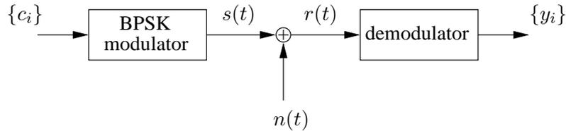
**Figure 2.3:** Simple channel model.
