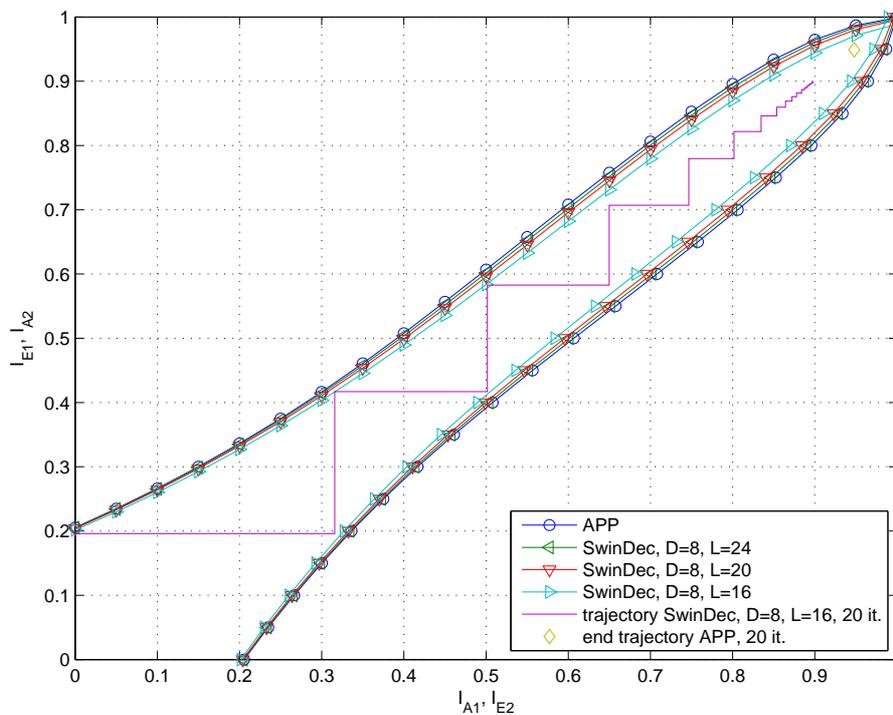
**Figure 5.30:** EXIT chart analysis of the (1932,640) UMTS turbo code decoded with different SwinDec component decoders at a  $E_b/N_0$  value of 0.5 dB.
