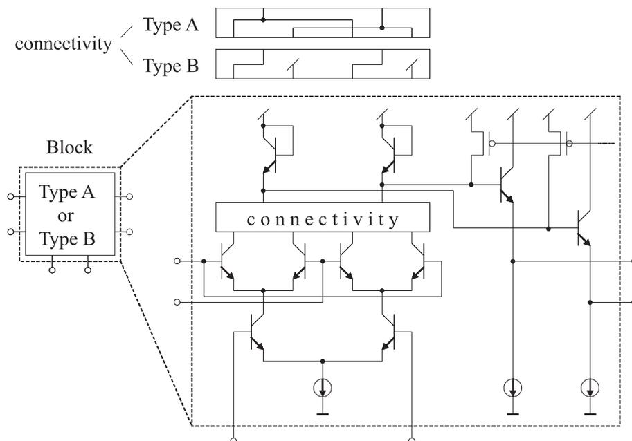
**Figure 7.10:** Decoder building block with connectivity for Type A and Type B blocks.
