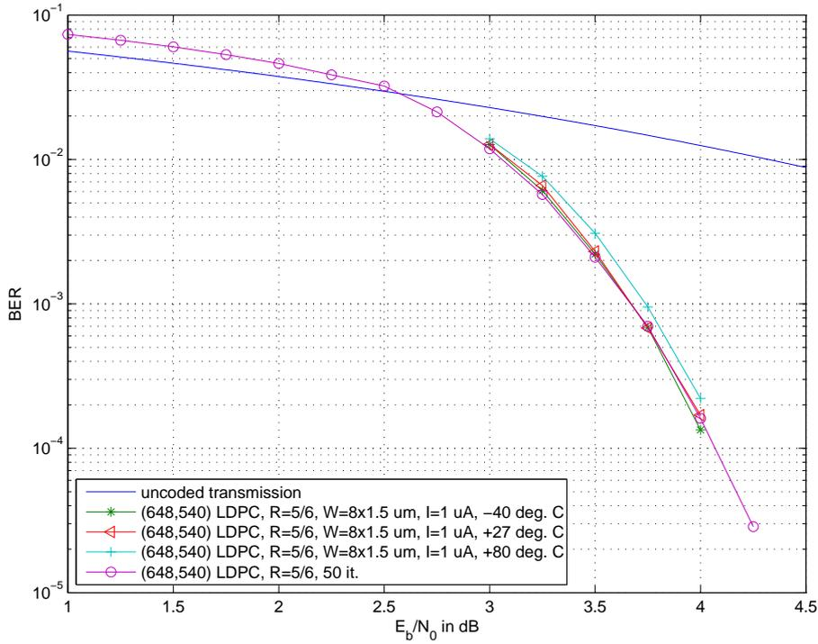
**Figure 8.12:** Estimated BER of the  $R = 5/6$  analog LDPC decoder at different temperatures (with trimming).
