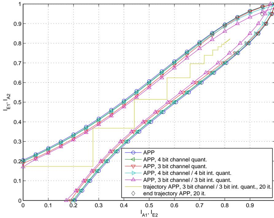
**Figure 5.32:** EXIT chart analysis of the (1932,640) UMTS turbo code decoded with different component decoders and quantization of soft information at a  $E_b/N_0$  value of 0.5 dB.
