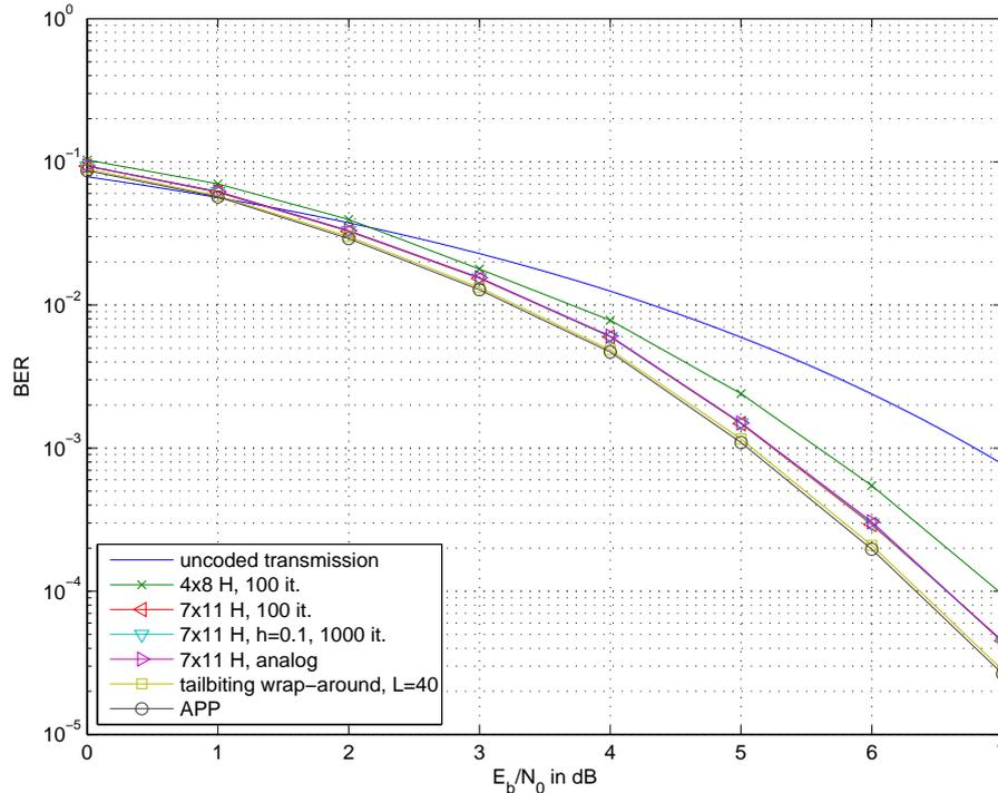
**Figure 5.12:** Decoding of the (8,4,4) extended Hamming code based on different code graphs.
