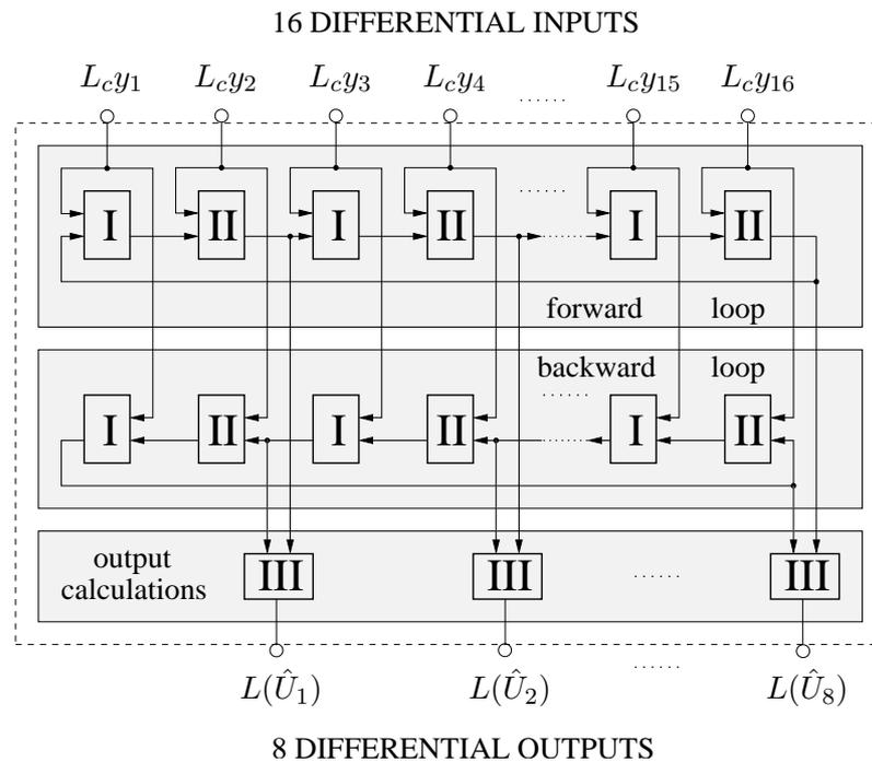
**Figure 7.6:** Block diagram of the BiCMOS decoder chip.
