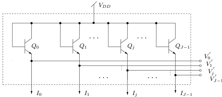
**Figure 6.9:** Inverse probability multiplexor ( $\text{pMUX}^{-1}$ ) consisting of diode-connected transistors.
