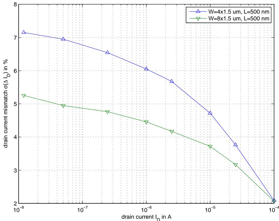
**Figure 8.16:** Drain current mismatch for nMOS transistors with different size.
