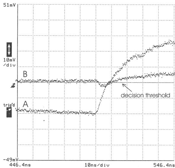
Figure 7.9: Measured transient response of the decoding network showing the correction of two bit errors.
