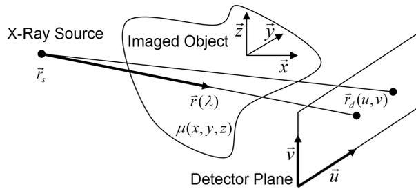
Figure A.1.: Scheme of X-Ray projection imaging
