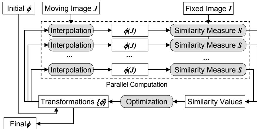
Figure 2.10.: Parallelized scheme of an image-based registration algorithm.
