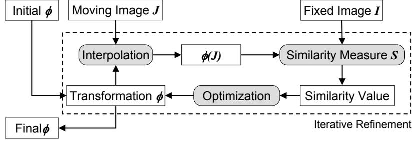
Figure 2.2.: Iterative scheme of an image-based registration algorithm.
