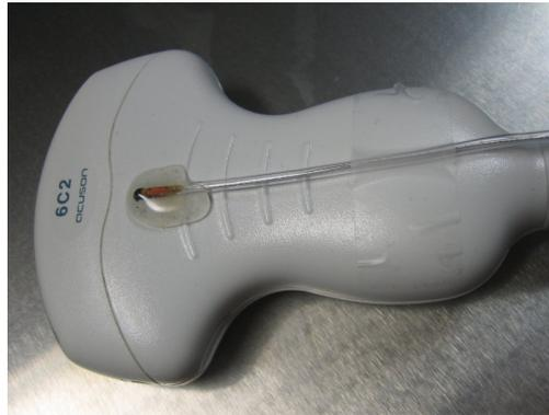
Figure 5.9.: Magnetic tracking sensor hot-glued onto the ultrasound probe.
