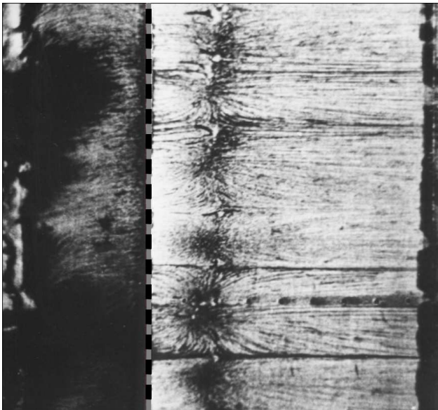
Figure 4.5: Oil-flow visualization pattern from higher-Reynolds-number experiment, the thick dashed vertical line indicates the corner position.
