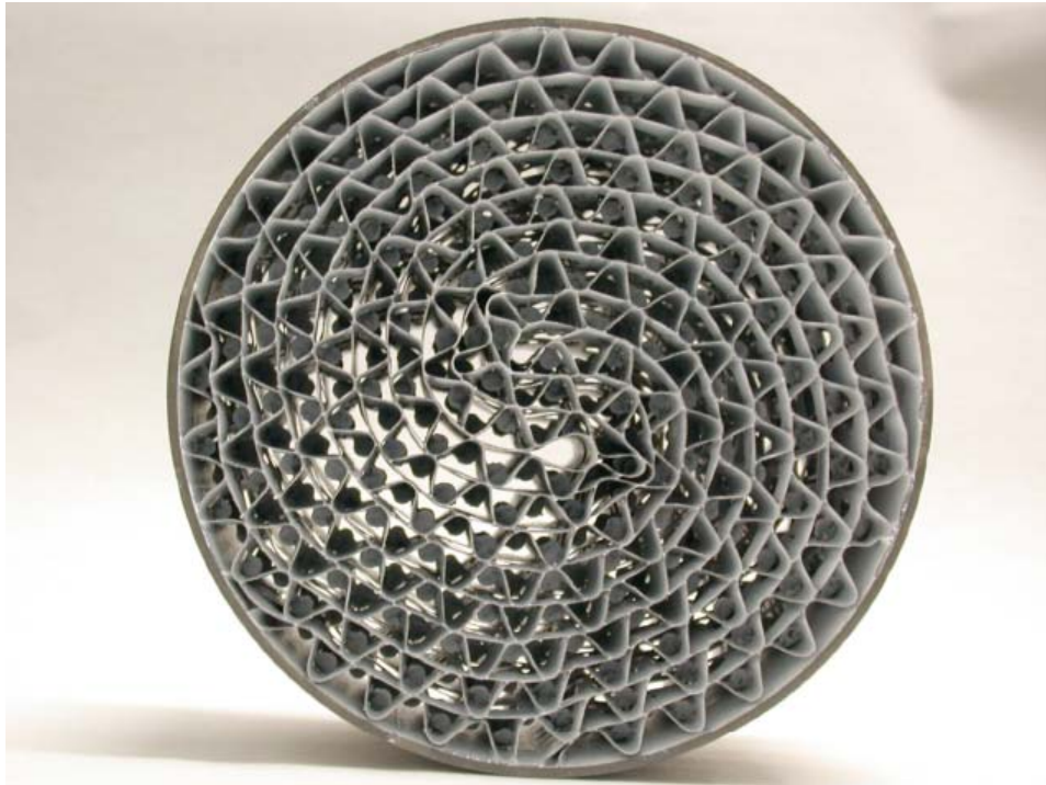
Figure 1.5 Transmitted light photograph of a coated H-cat with special mixing structure [53].
