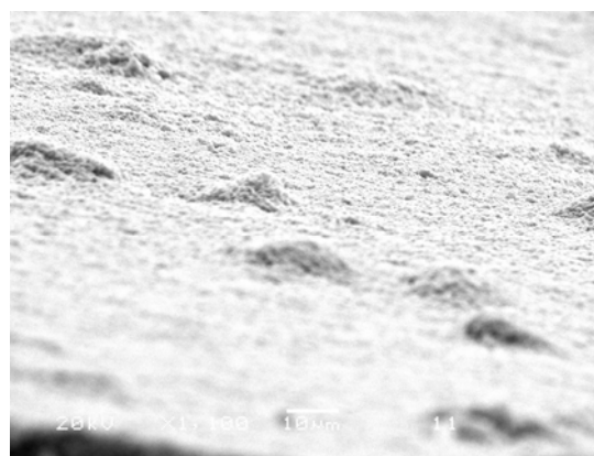
Figure 4.14 SEM picture 2 of catalyst #1 with thin coating thickness.
