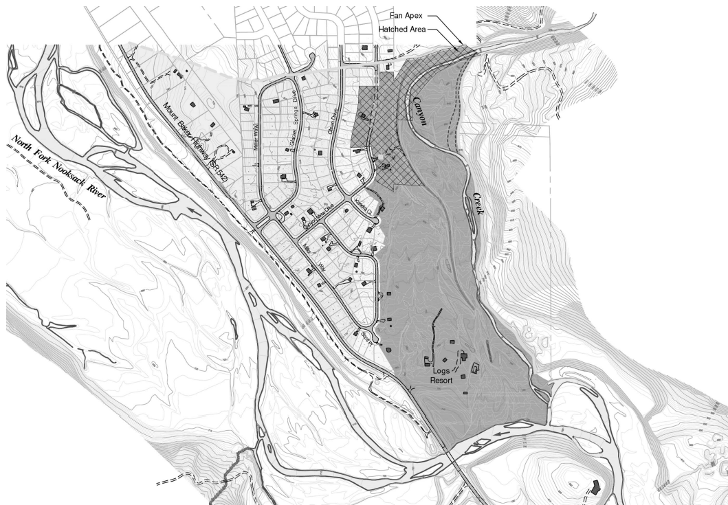
Figure 7.1: Hazard zoning at the alluvial fan of Canyon Creek, from Jakob et al. [52]
