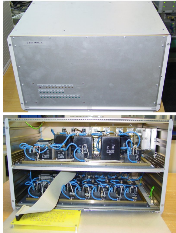
Figure 2.25: The MIRA capacitance adaptation boxes (C-boxes). The mica capacitors are connected in parallel and suited for high voltage.
