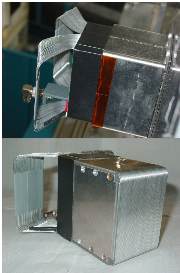
Figure 2.20: The MIRA coupling coils are mounted at the front sides of the shieldings inside a Mu-metal nozzle. It implements an abrupt field transition on one side, and an adiabatic on the other.
