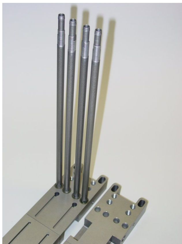
Figure 2.9: The top and bottom panels with inserted cooling pipes. Waterproof mounting is achieved by an o-ring seal.
