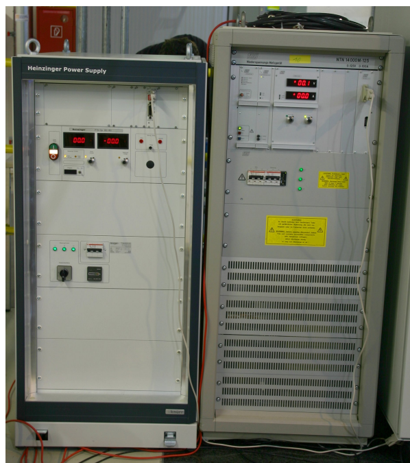
Figure 2.26: DC power supplies: Heinzinger PTN 3p 80-80 (left) and FUG NTN 14000M-125 (right).
