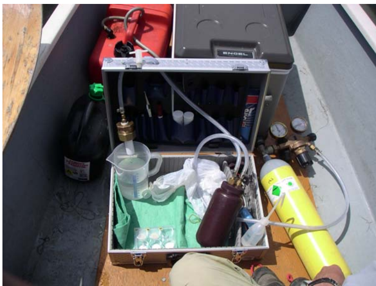
Figure 4.4: Filtration set up on the boat
