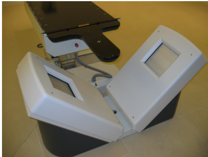
Figure 7.2: The detectors of the stereo X-ray imaging of the Cyberknife ® Radiosurgical System.
