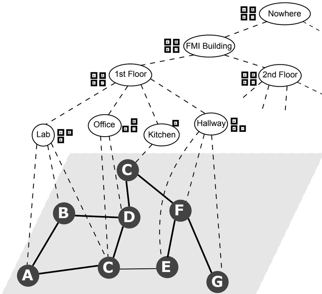
Figure 6.9: Hierarchical reduction of configuration data. At every hierarchical step, new sets of object descriptions are used.
