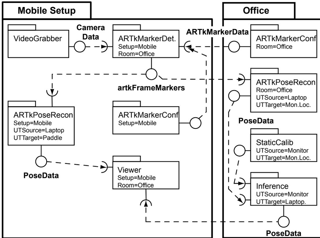
Figure 7.5: DWARF components involved in runtime spatial data flow. This UML diagram shows a representative part of the system state in location Office.
