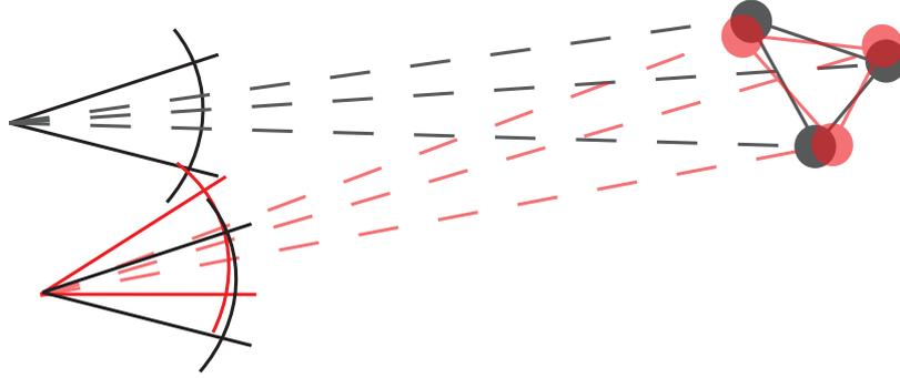
Figure 3.1: Why the SR graph needs to be directed: If the object’s real state (black) is measured with some error (red), the positional accuracy remains high, while the orientational accuracy degrades. If we look at the situation from the object’s perspective and want to estimate the camera’s pose in the object’s coordinate system, the positional accuracy degrades, while the orientational accuracy is high.
