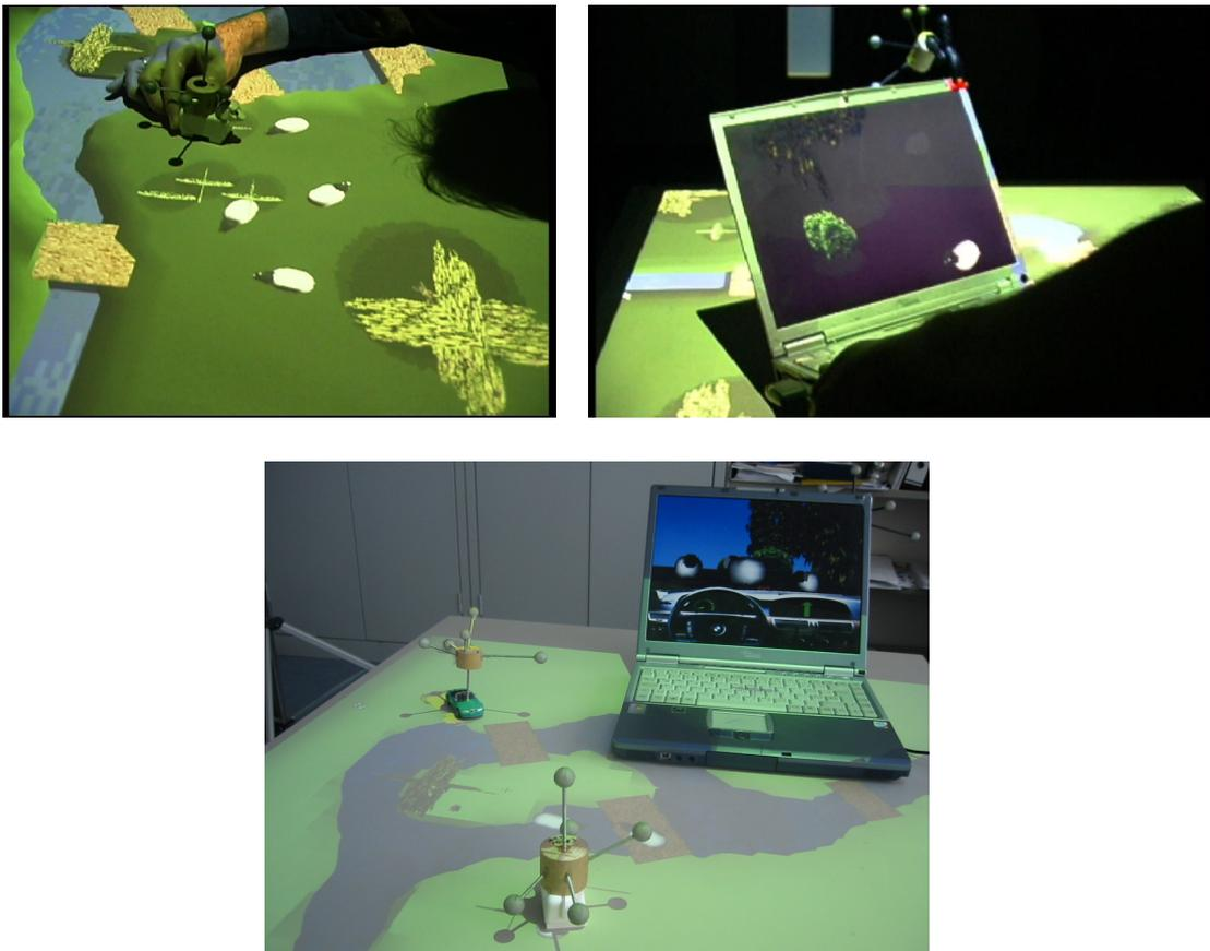
Figure 3.15: Pictures of the SHEEP game. On the top left, a player moves the tangible sheep, and the herd of virtual sheep follows it. On the top right, a spectator uses a laptop to view the scenery in three dimensions. The bottom image shows the view through a tracked car's windscreen.
