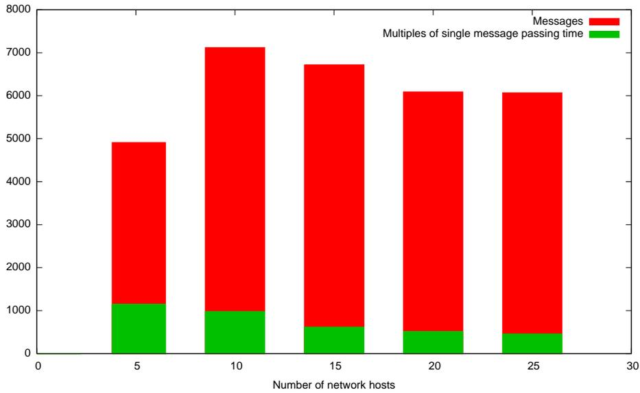
Figure 4.4: Simulation result with number of network hosts as a parameter. The underlying graph had 50 vertices and on average 5 pairs of edges adjacent to every vertex.
