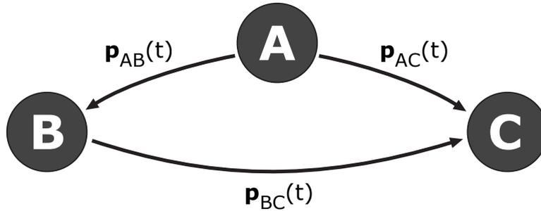
Figure 3.3: Measurement Graph  $G(\Phi)$ : An edge between two nodes only exists if a measurement of the spatial relationship of the objects they represent has been made.
