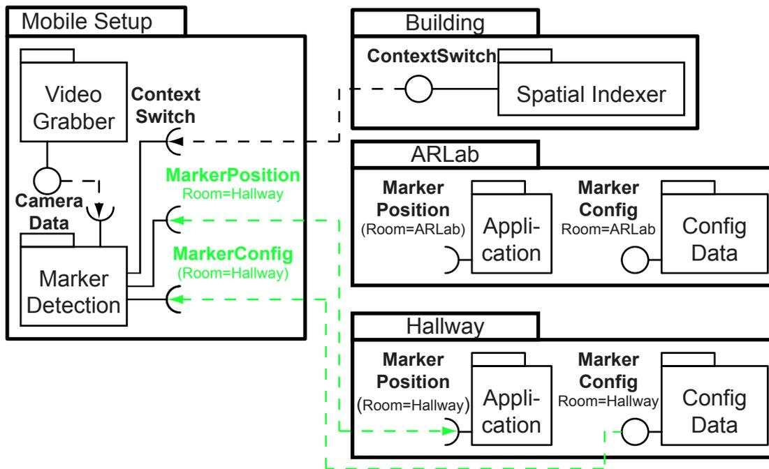
Figure 6.3: Example setup after configuration change. The marker detection service changed its ability attributes and need predicates such that it gets a new configuration from the hallway's corresponding service and sends its data to another application.
