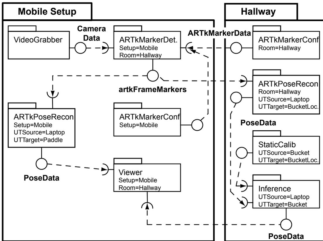
Figure 7.6: DWARF components involved in runtime spatial data flow. This UML diagram shows a representative part of the system state in location Hallway.
