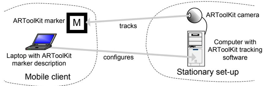
Figure 6.8: A mobile locatable is to be identified by a stationary camera. Thus, the mobile setup has to transmit information about the locatable to the stationary environment. (Taken from [114].)
