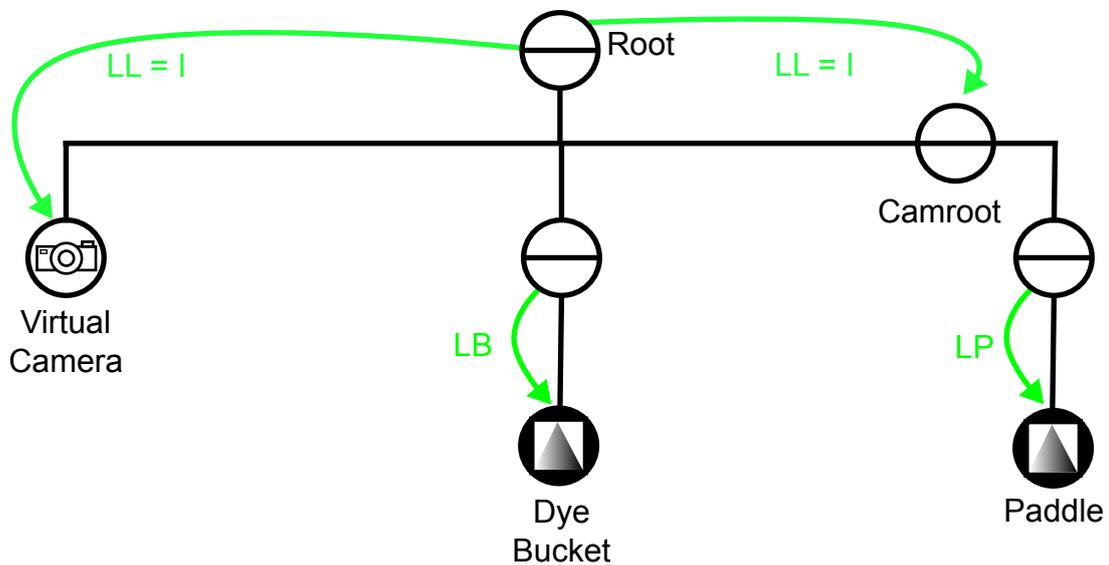
Figure 7.9: Hallway location scene graphs shown in DWARF Viewer. The camera is modeled as stationary, thus its pose relative to the root of the scene graph is identity. Both the bucket's and the paddle's poses are set based on ARToolkit measurements.
