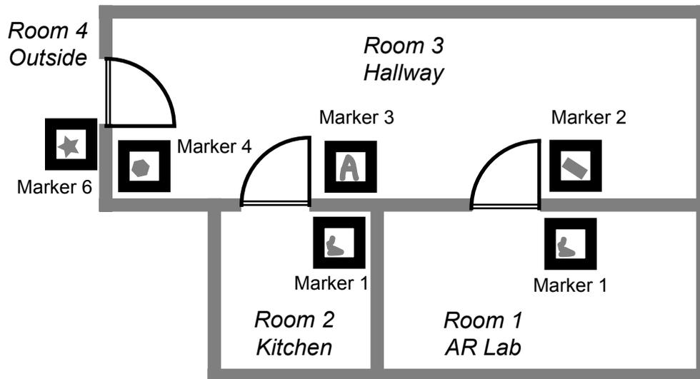
Figure 6.4: Physical setup of ARCHIE scenario. Note that the ARToolkit markers used for spatial indexing can be reused, the outgoing marker both in the ARLab and the kitchen are identical.
