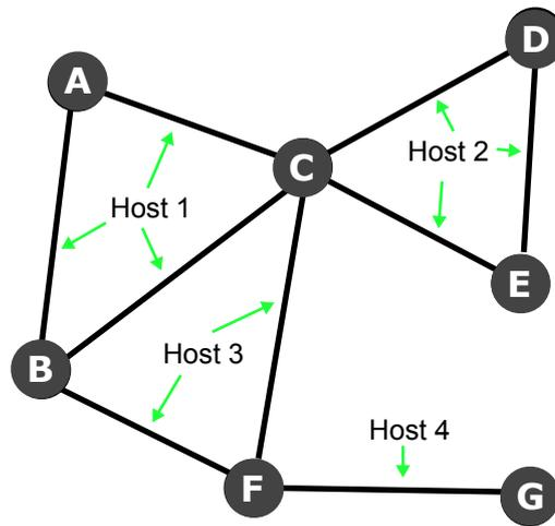
Figure 4.1: A spatial relationship graph describing a distributed sensor network. Every edge corresponds to some software component delivering interpreted data from some sensor. Every software component is executed on some host in the network.
