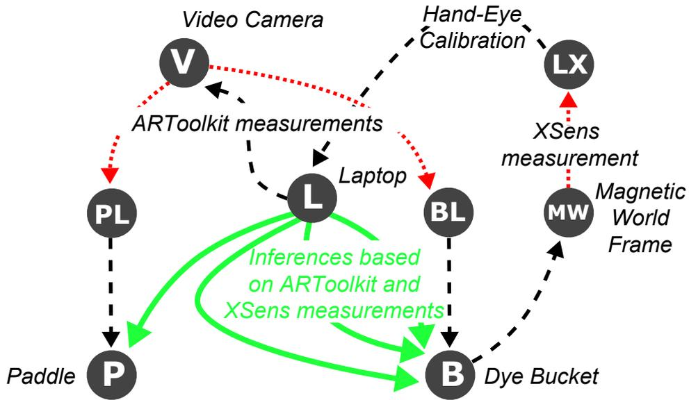
Figure 7.3: SR graph of hallway setup. The laptop needs the relative pose of the paddle and the dye bucket, in addition, collisions between these two objects have to be detected.
