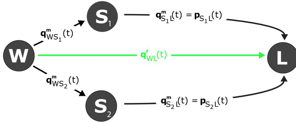
Figure 3.9: Modeling complementary sensor fusion in the Ubitrack formalism.
