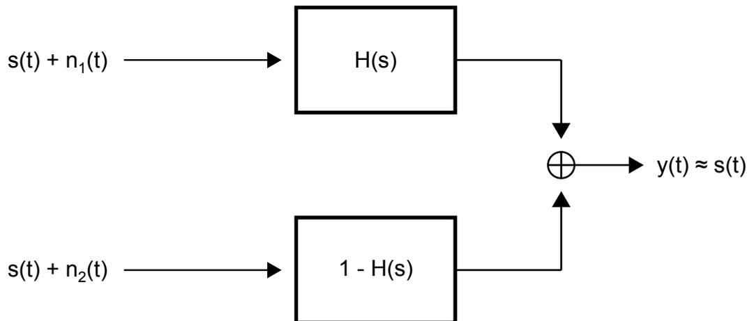
Figure 2.1: A complementary filter for two measurements (taken from [11]).
