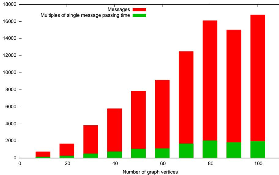
Figure 4.5: Simulation result with number of graph vertices as a parameter. The random graph had on average 5 pairs of edges adjacent to every vertex and was distributed on 10 hosts.
