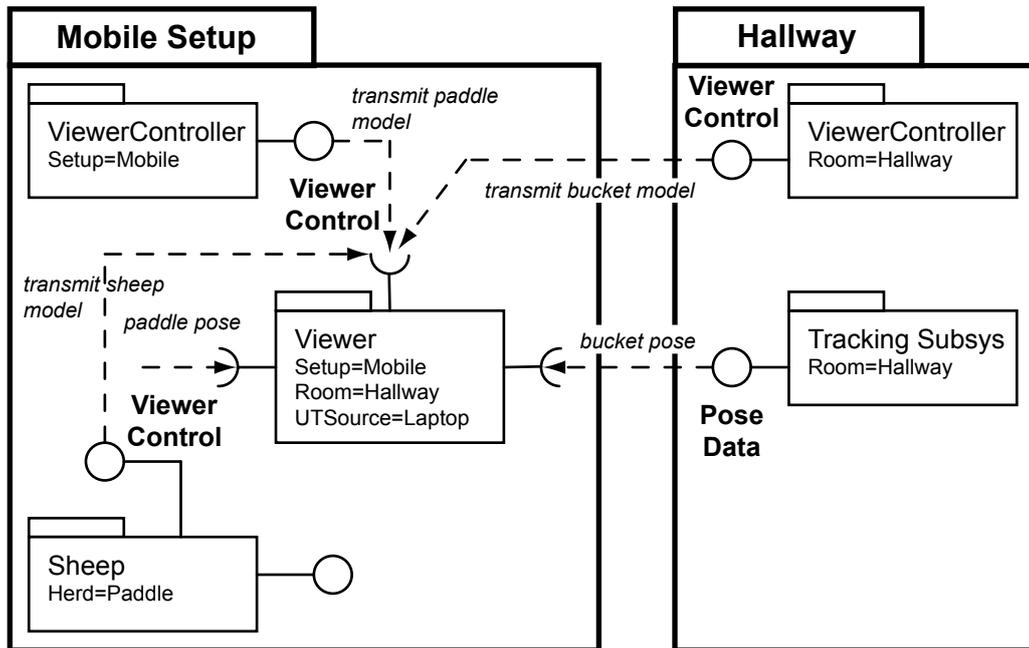
Figure 7.11: DWARF components involved in runtime reconfiguration of the mobile setup’s Viewer. This UML diagram shows the system state in location Hallway.
