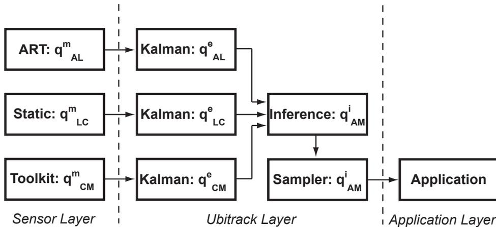
Figure 5.7: DWARF data flow components of extended tracker range example. The diagram shows the SR graph functions corresponding to the individual services and the logical layering of the services. Arrows indicate the data flow.
