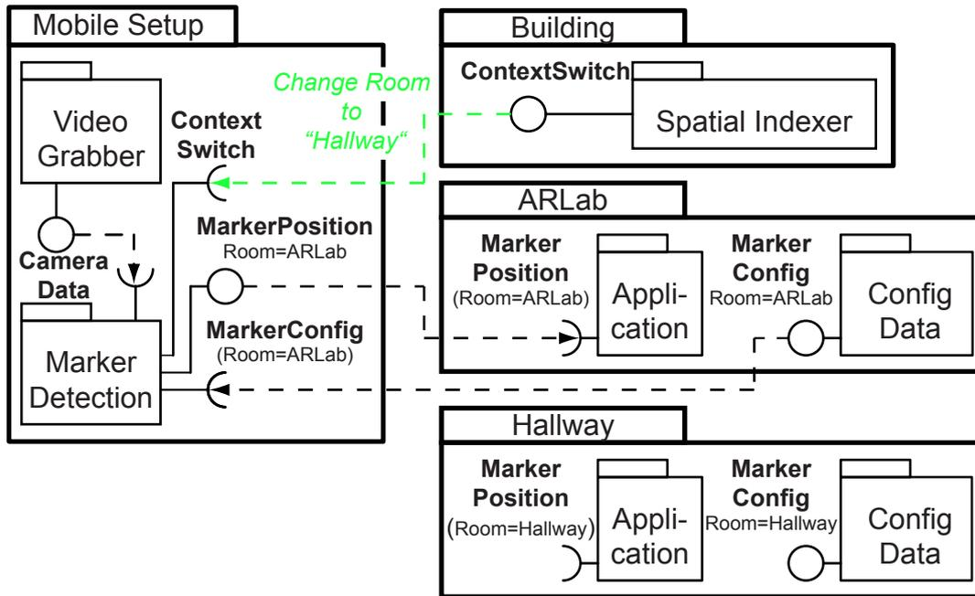
Figure 6.2: Example setup. The spatial indexer notices that the user carrying the mobile setup leaves the AR lab and goes to the hallway. It sends a corresponding event to all interested services on the mobile setup.
