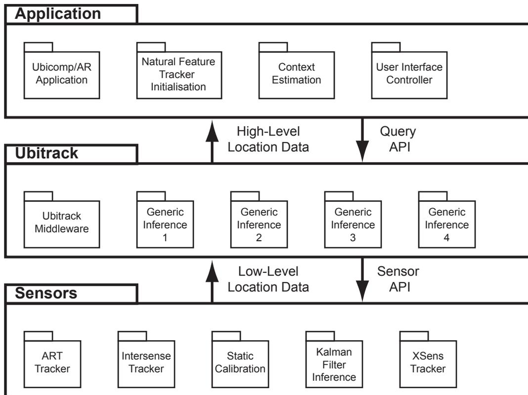
Figure 5.5: Layered Ubitrack architecture. The Ubitrack layer is an abstraction from the low-level location sensors and provides a powerful API to arbitrary applications.
