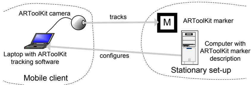
Figure 6.7: A stationary locatable is to be identified by a mobile camera. Thus, the stationary environment has to transmit information about the locatable to the mobile setup. (Taken from [114].)
