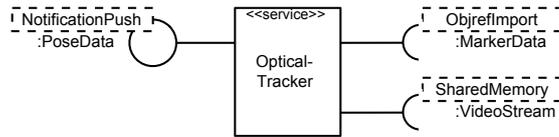
Figure 5.2: Sample UML description of an optical tracker service. Needs are depicted as semicircles, abilities as circles.
