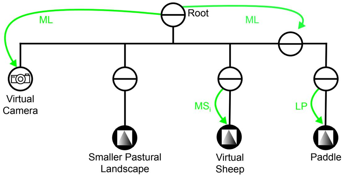
Figure 7.8: Office location scene graph shown in DWARF Viewer. Again, the pastoral landscape is stationary. The pose of the virtual sheep is set by the simulation, and both the camera's and the paddle's pose are set by inferences based on ARToolkit measurements.
