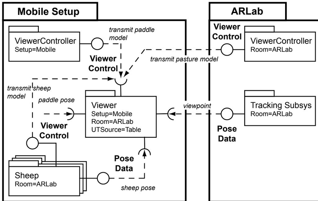
Figure 7.10: DWARF components involved in runtime reconfiguration of the mobile setup’s Viewer. This UML diagram shows the system state in location ARLab.
