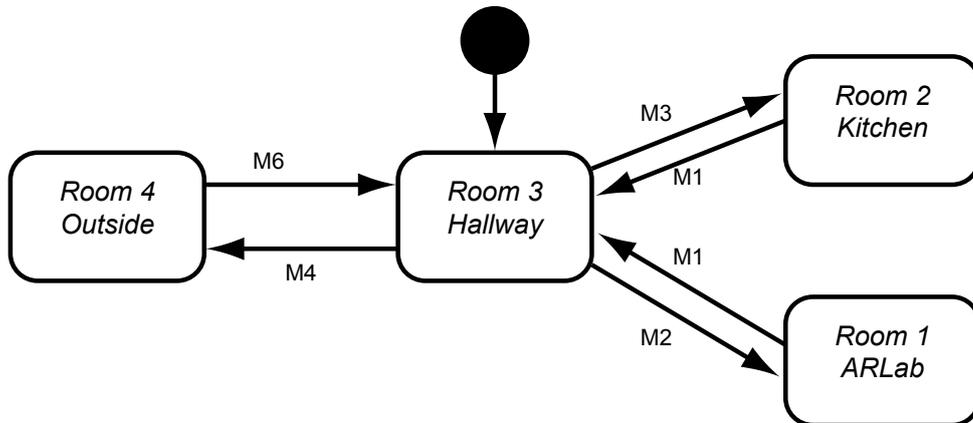
Figure 6.5: State transition diagram of ARCHIE spatial indexer.
