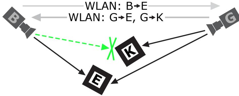
Figure 3.12: Shared optical tracking setup: Two cameras try to detect the pose of two markers. Missing information is exchanged over a wireless network.
