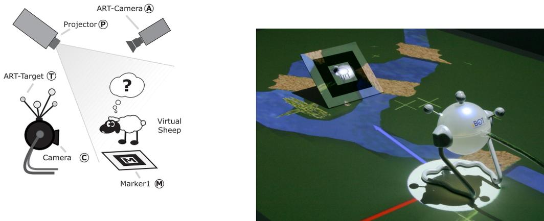
Figure 3.10: Extended tracker range setup: An ART system tracks a camera that detects a fiducial marker outside the ART system's range. This information gets used to project a virtual sheep onto the marker.
