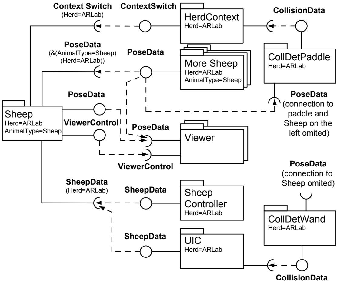
Figure 7.12: DWARF components involved in runtime virtual sheep reconfiguration if the sheep is in herd state ARLab or Monitor.
