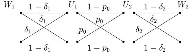
**Figure 4.5:** Binary symmetric test channels. We can view the correlated binary sources  $U_1$  and  $U_2$  as the input and the output of a binary symmetric channel with crossover probability  $p_0$ . The auxiliary random variables  $W_1$  and  $W_2$  can be obtained likewise using two test channels with crossover probabilities  $\delta_1$  and  $\delta_2$ , respectively.
