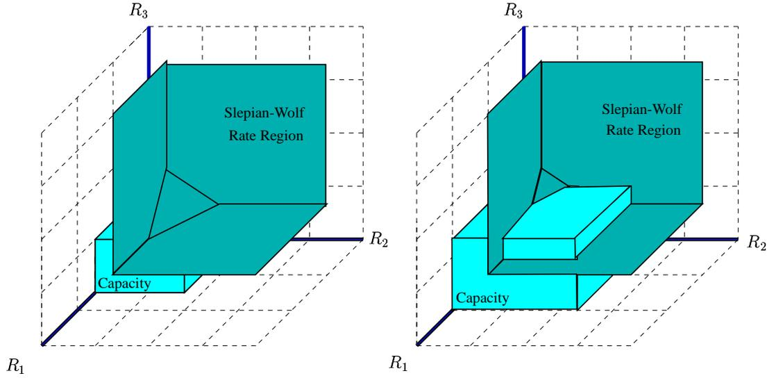
**Figure 3.8:** A sketch of the regions involved in Theorem 3.5 for  $M = 3$  sources. Once again, when the capacity region of the independent reachback channels does not intersect the Slepian-Wolf rate region (left plot) reliable communication is not possible. If the two regions do intersect (right plot) then all points in the intersection are achievable.
