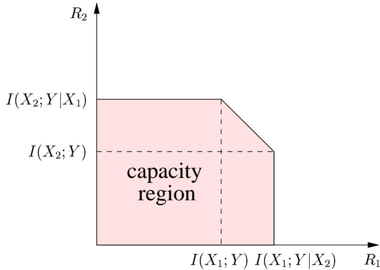
**Figure 2.8:** The capacity region of the multiple access channel.
