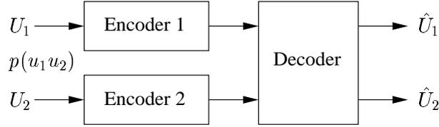
**Figure 4.1:** System setup for the multiterminal source coding problem.
