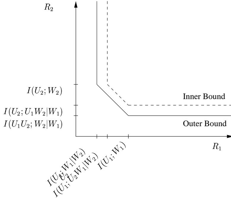
**Figure 4.4:** Our rate-distortion inner bound in comparison to the Berger-Tung outer bound for a fixed value of  $(D_1, D_2)$ .
