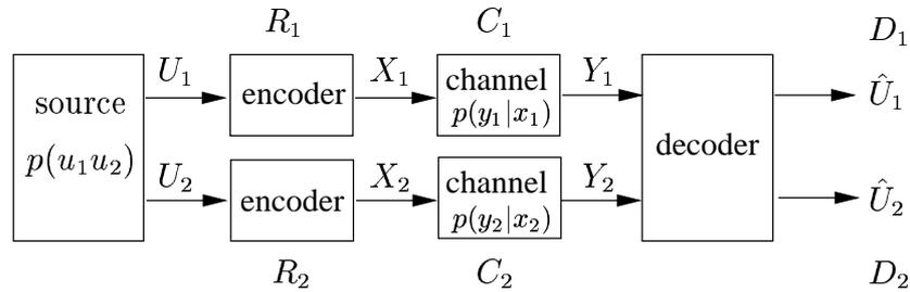
**Figure 4.2:** A rate-distortion version of the sensor reachback problem.
