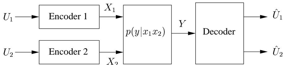
**Figure 2.7:** The multiple access channel.
