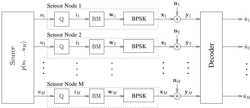
**Figure 5.1:** System model.  $M$  correlated samples are separately encoded by  $M$  sensor nodes, consisting of a scalar quantizer, a bit mapper and a modulator. The data is then transmitted over an array of independent AWGN channels and decoded jointly at the receiver.
