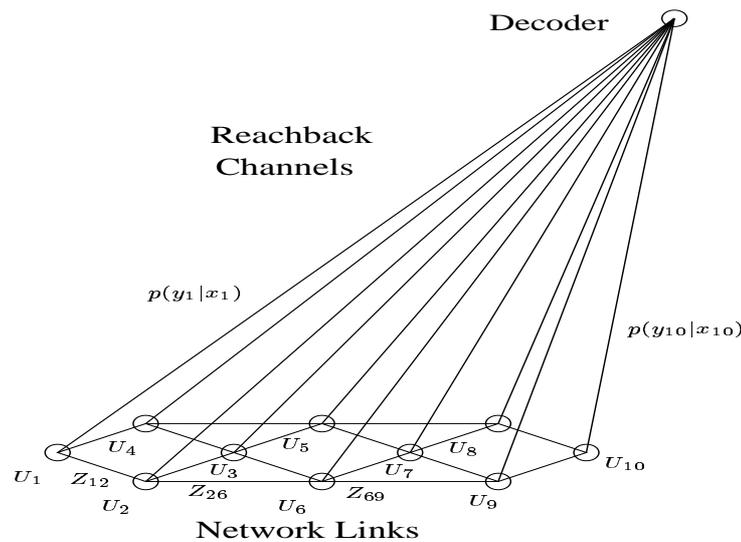
**Figure 3.9:** Reachback communication with  $M \geq 2$  partially cooperating nodes.
