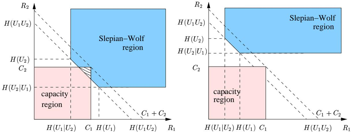
**Figure 3.4:** Relationship between the Slepian-Wolf region and the capacity region for two independent channels. In the left figure, as  $H(U_1|U_2) < C_1$  and  $H(U_2|U_1) < C_2$  the two regions intersect and therefore reliable communication is possible. The figure on the right shows the case in which  $H(U_2|U_1) > C_2$  and there is no intersection between the two regions.
