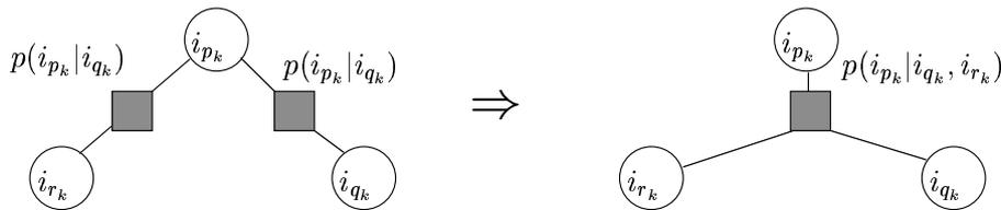
**Figure 5.8:** The basic procedure in Algorithm 5.5 consists of replacing two degree-2 function nodes by one degree-3 function node. The replacements are chosen according to the associated reduction of the KLD.
