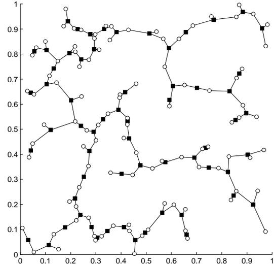
(b)  $M = 100$  sensors**Figure 5.9:** Degree-3 factor trees for  $M$  sensors placed randomly on the unit square, according to the source model described in Section 5.2.1.
