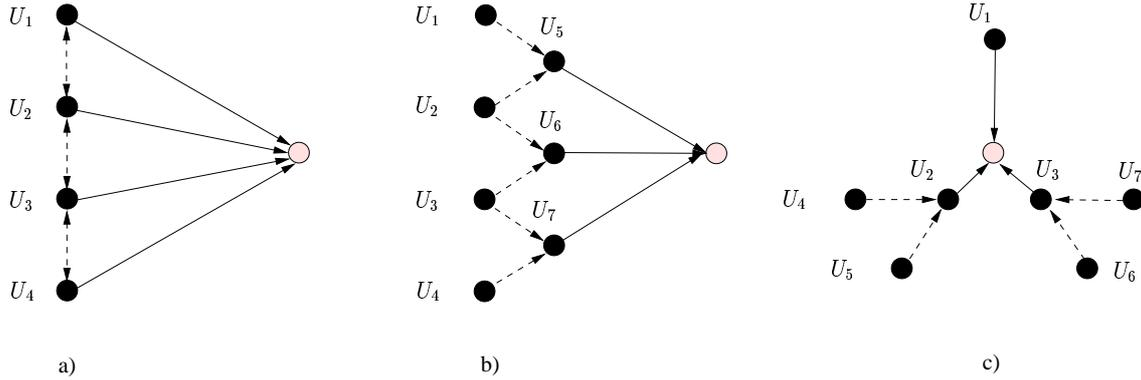
**Figure 3.10:** Three sensor network topologies for which Theorem 3.7 gives the reachback capacity. Dark circles denote the sensor nodes and a light circle represents the remote receiver. Conference channels and reachback channels are depicted as dashed and solid arrows, respectively, with the arrow head indicating the direction of the flow of information. Conferencing is done before transmission over the reachback channels.
