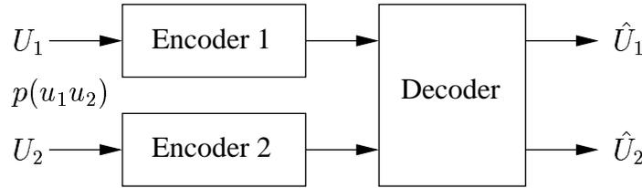
**Figure 2.5:** Separate encoding of correlated sources (*Slepian-Wolf problem*). The noiseless channels between the encoders and the decoder are omitted.
