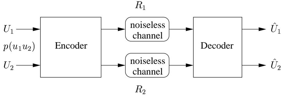
**Figure 2.4:** Joint encoding of correlated sources.
