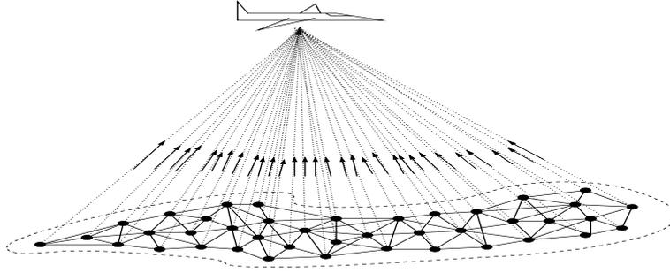
**Figure 3.1:** A large number of sensors is deployed over a target area. After collecting the data of interest, the sensors must *reach back* and transmit this information to a single receiver (e.g., an overflying plane) for further processing.
