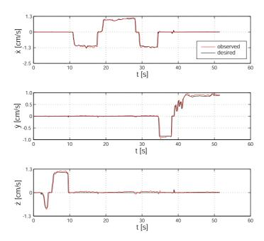
Figure 3.4: Velocity of TCP, desired and observed.
