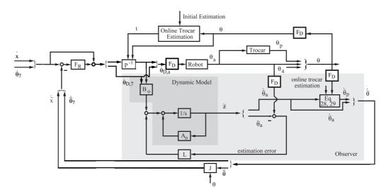
Figure 3.2: Velocity control structure.
