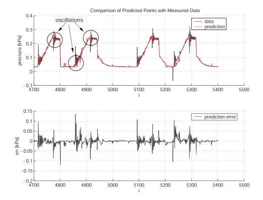
Figure 5.8: Good prediction of RPS. Parameters:  $f_{\text{sample}} = 40 \text{ Hz}, s = 1, M = 10, p=10, h=20, \bar{n} = 4700, n = 5400.$
