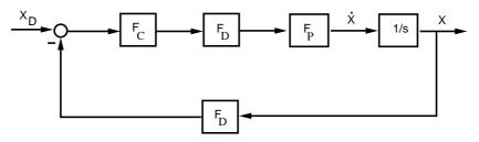
Figure 3.12: Closed control loop.
