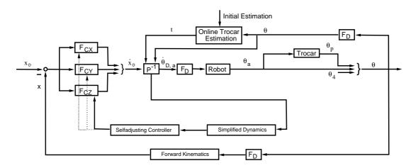
Figure 3.17: Position control scheme.
