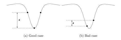
Figure 4.22: Global minimum between grids of the CCD chip [69].
