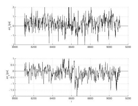
Figure 5.27: Prediction error using ECG and RPS. Parameters:  $\xi = 1.0 \frac{\text{kPa}}{\text{mV}}$ , s=1, p=56, h=18, M=8,  $\bar{n} = 4000$ , n=8100.
