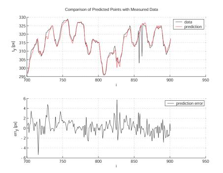
Figure 5.11: Prediction of HST with outlier detection. Parameters:  $f_{\text{sample}} = 25 \text{ Hz}, s = 1, M = 10, p=7, h=4, \bar{n} = 700, n = 900.$
