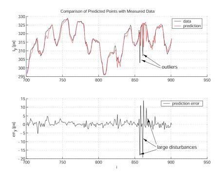
Figure 5.10: Prediction of HST without outlier detection. Parameters:  $f_{\text{sample}} = 25 \text{ Hz}, s = 1, M = 10, p=7, h=4, \bar{n} = 700, n = 900.$
