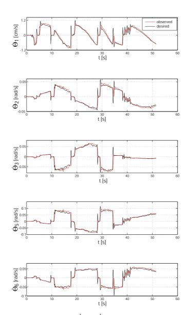
Figure 3.6: Velocities  $\dot{\Theta}_1$  ..  $\dot{\Theta}_6$ , desired and observed.
