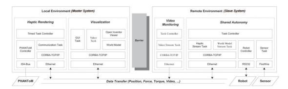
Figure 2.12: Distributed master-slave system architecture.
