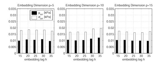
Figure 5.9: Evaluation of  $\mu_{\text{err}}$  and  $\sigma_{\text{err}}$  for different *p*-*h*-combinations. Parameters:  $f_{\text{sample}} = 40 \text{ Hz}, s = 1, M = 10, \bar{n} = 4700, n = 5400.$
