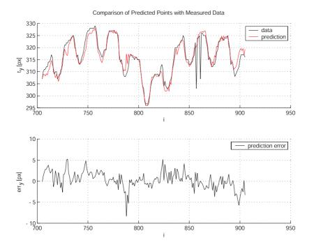
Figure 5.13: Five-step prediction of HST with outlier detection. Parameters:  $f_{\text{sample}} = 25 \text{ Hz}, s = 5, M = 10, p=12, h=2, \bar{n} = 700, n = 900.$
