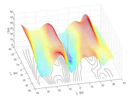
Figure 4.21: SSD measure versus  $t_x, t_y$  at LM2 (applied to same image).
