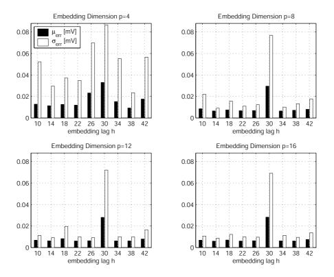
Figure 5.5: Evaluation of  $\mu_{\text{err}}$  and  $\sigma_{\text{err}}$  on a simulated ECG with  $f_{\text{ECG}} = 80$  bpm for different p and h. Parameters:  $f_{\text{sample}} = 80$  Hz, s=1, M=10,  $\bar{n}=3680$ , n=4370.
