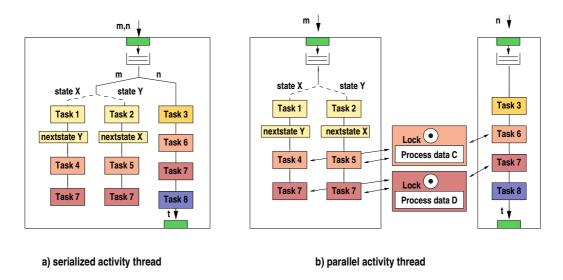
Figure 4.8: Activity thread model alternatives
