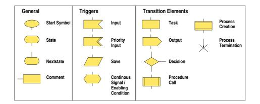
Figure 3.2: SDL-92 EFSM Elements
