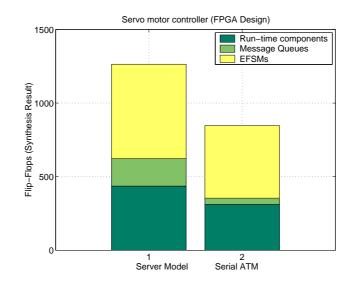
Figure 7.9: Servo controller: memory elements of the entire FPGA design
