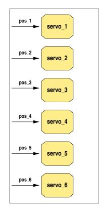
Figure 7.4: SDL specification of the servo motor controller
