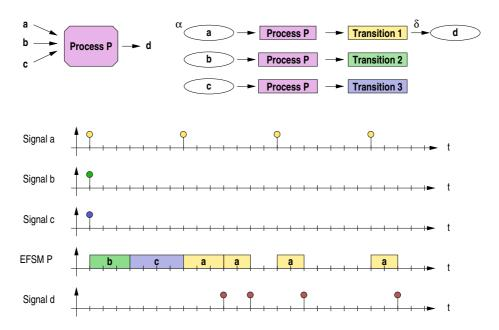
Figure 5.10: Example for internal signal d
