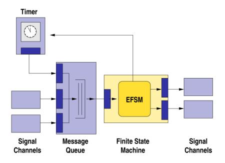
Figure 4.2: Basic hardware architecture implementing one SDL process
