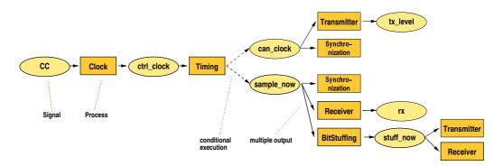
Figure 7.15: Task precedence system triggered by signal CC
