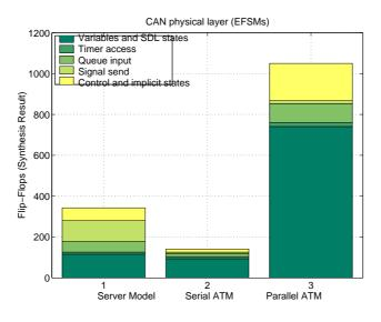
Figure 7.8: CAN bus: memory elements of the EFSM implementation
