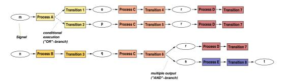
Figure 4.6: Task precedence graph of the SDL system from figure 4.4
