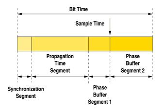
Figure 7.1: Internal bit timing in CAN
