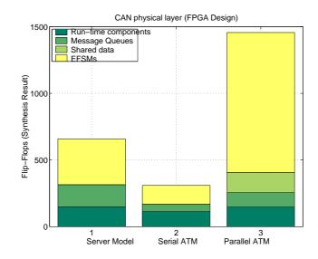
Figure 7.7: CAN bus: memory elements of the entire FPGA design
