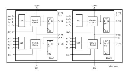
Figure 7.13: Xilinx Virtex configurable logic block consisting of two slices
