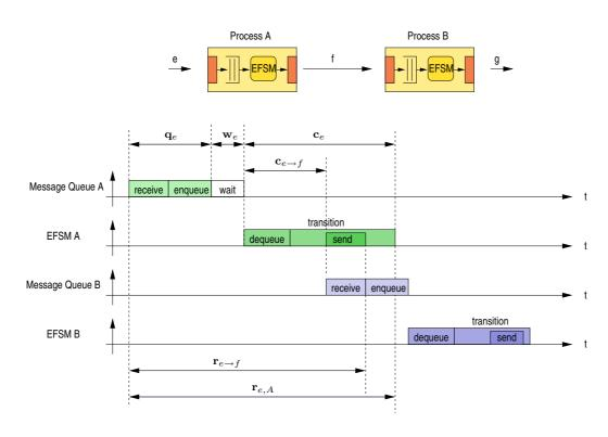
Figure 5.2: Timing relationship in a precedence system
