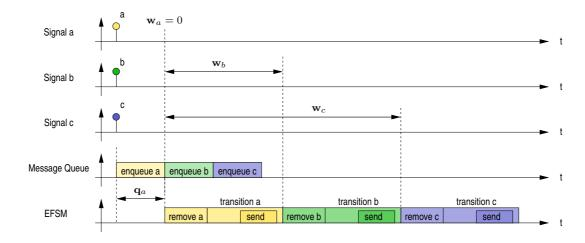
Figure 5.5: Detailed view of the waiting time
