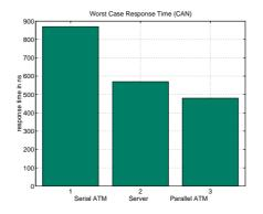
Figure 7.18: Maximum response time for the CAN bus example
