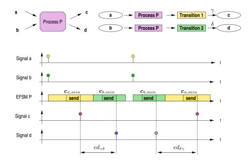
Figure 5.13: Event dependencies between signals from one SDL process (different transitions)
