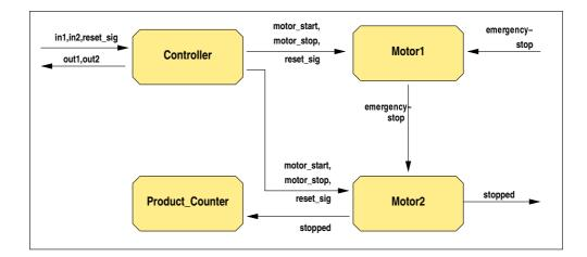
Figure 7.5: SDL specification of the assembly line example
