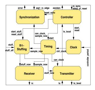
Figure 7.2: SDL specification of the CAN physical layer (SDL processes)
