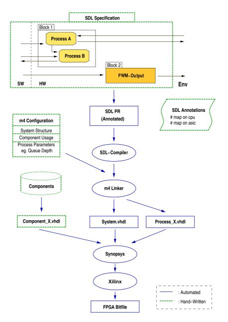
Figure 6.5: Rapid prototyping hardware design process
