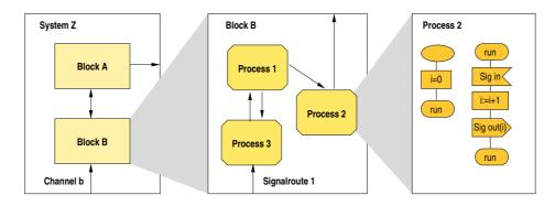
Figure 3.1: Example SDL System Structure
