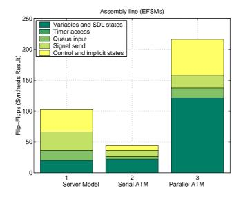
Figure 7.12: Assembly line: memory elements of the EFSM implementation
