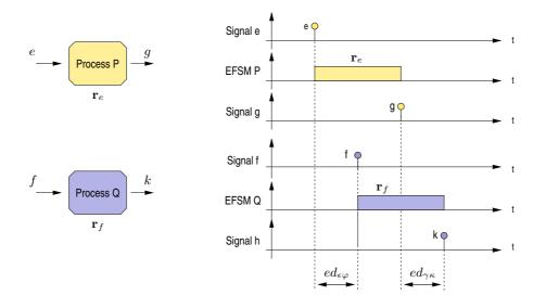
Figure 5.15: Propagation of event dependencies between SDL processes
