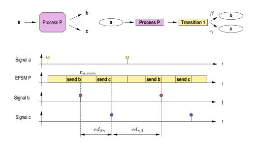
Figure 5.14: Event dependency between signals from one SDL process (one transition)
