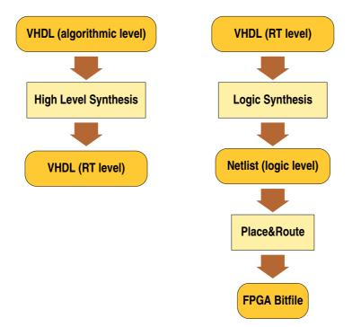
Figure 4.1: Hardware design flow targeting FPGA
