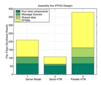
Figure 7.11: Assembly line: memory elements of the entire FPGA design
