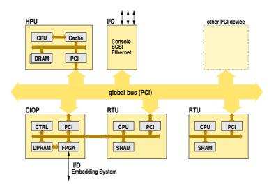
Figure 6.1: Rapid prototyping target architecture – block diagram
