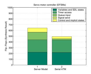
Figure 7.10: Servo controller: memory elements of the EFSM implementation
