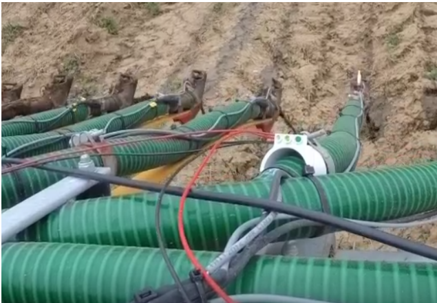
Fig. 11. A photo showing a white clip holding three LEDs on the hose. The LEDs flash when the section is turned on, aiding with time-synchronising the camera video with the data logged from the CAN bus.
