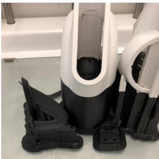
Fig. 7. A photograph showing the 3D printed slurry shoes.
