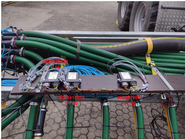
Fig. 2. Axiomatic A/D Converter mounted at the boom. The Axiomatics read the input voltages and writes them out as ISO 11783 proprietary CAN frames.
