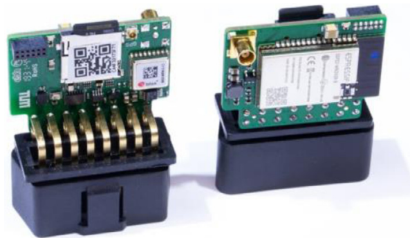
Fig. 8. The data logger developed at the Institute of Automotive Engineering, featuring an ESP-32 microcontroller, a MAX-M8W GNSS module by ublox and an external GNSS Antenna.
