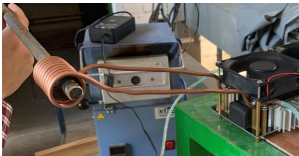
Figure 2: Induction coil to heat steel reinforcement.
