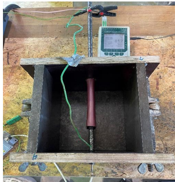
Figure 4: Measuring the Temperature on the rebar surface while heating with heat cartridge.
