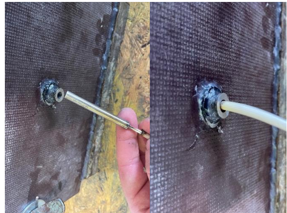
Figure 3: Heating cartridge being inserted into a pre-drilled rebar embedded in the pull-out test setup
