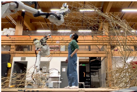
(a) Improv-Structure : humans and robotic arms collaboratively assemble an unplanned bamboo rod structure [36]
