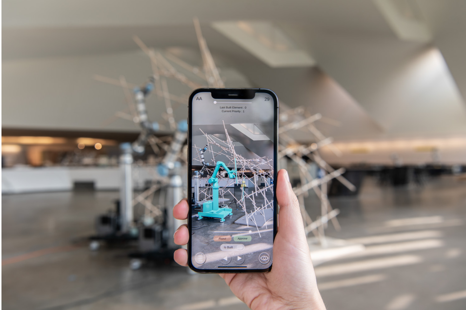
Figure 4.53: The custom AR phone-based application serves as a communication interface between the cooperating agents - human and robots - in the assembly process
