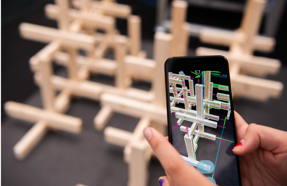
Figure 4.17: The visual display of the AR device can superimpose cues on the real world video stream designed to assist the builders with information, in this particular case with visual cues on the design space in which they can make their design choices
