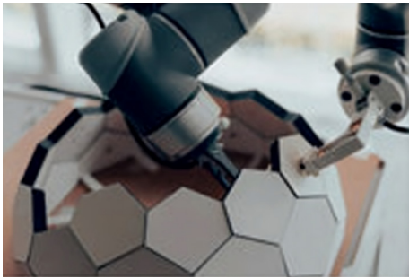
(c) Multi-robotic assembly of discrete shell structures [29]
