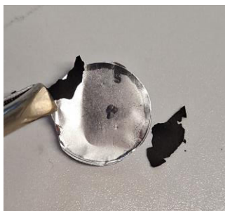
Figure 4-19: LFP cathodes with different catholytes and binders and the corresponding adhesion to the Al-foil. a PVDF ( M_w = 275 \text{ kg mol}^{-1} ), b Solef® 5130 PVDF.
