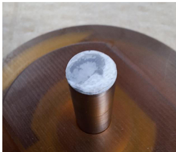
Figure 8-25: PEO-SPE film after a pressure test in the ASC-T cell. Clear indentation visible due to uneven pressure distribution in the cell setup.
