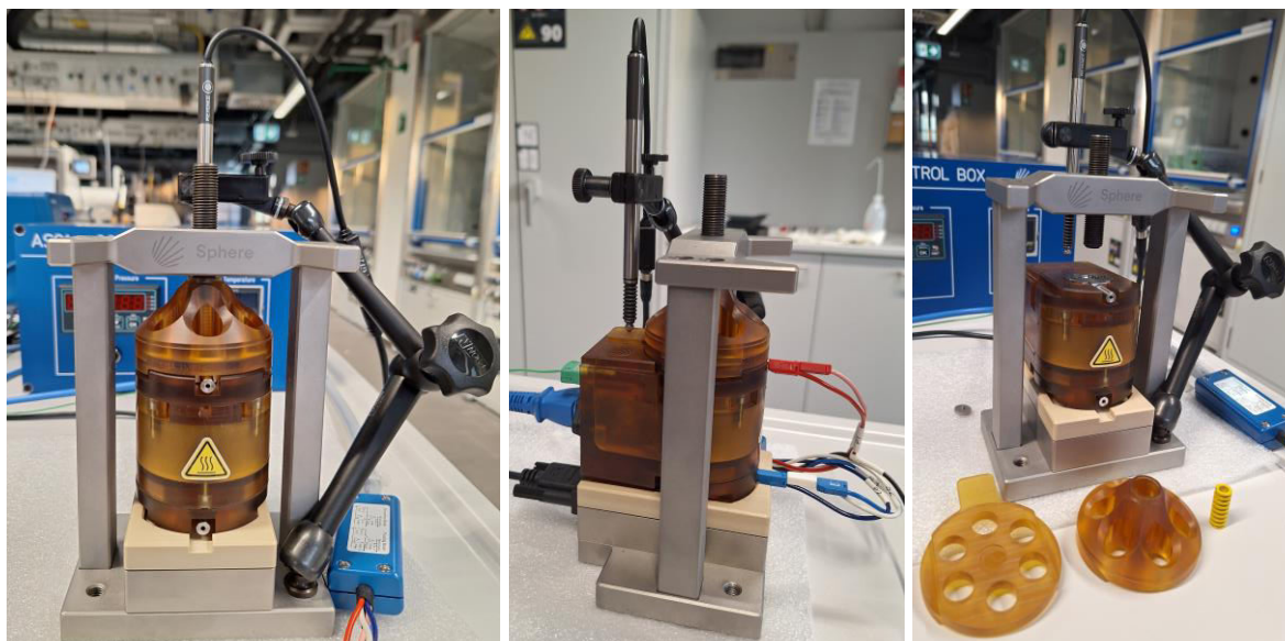
Figure 4-27: ASC-T cell in a constant pressure setup for monitoring thickness (and pressure) during electrochemical measurements. The thickness is measured by a sensor positioned on a platform, which is connected to a spacer between the top cell piston and the spring/screw to apply a specific pressure.
