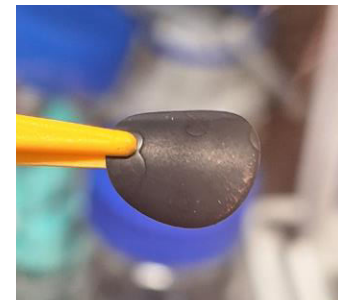
Figure 4-19: LFP cathodes with different catholytes and binders and the corresponding adhesion to the Al-foil. a PVDF ( M_w = 275 \text{ kg mol}^{-1} ), b Solef® 5130 PVDF.
