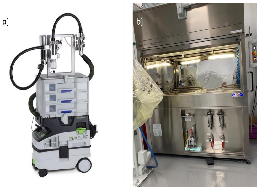
Figure 3: Particle extraction systems. a) Particle suction extraction system C|PS 2 by CleanControlling Technical, Dresden, Germany [69]. b) Cleanliness cabinet by PALL, New York USA. [Image by M. K. Lanzinger]
