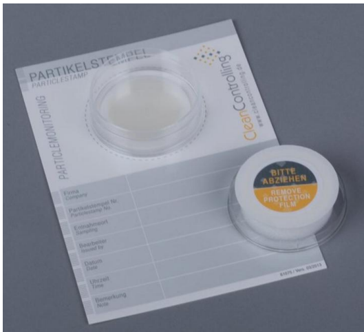
Figure 2: An example for a particle stamp used for sampling of surfaces for TCA from CleanControlling. [68]
