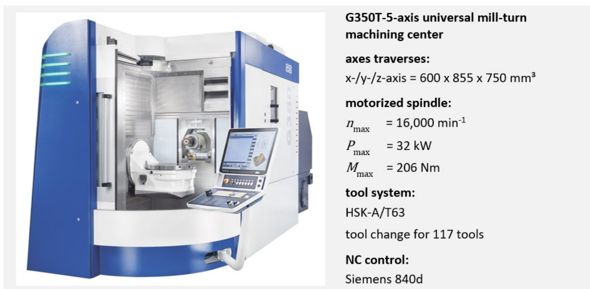
Figure 5-1: Specifications of the 5-axis universal mill-turn machining center Grob G350T
