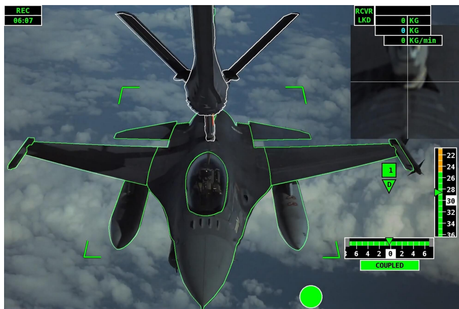
Figure 5-3: Visual air-to-air refuelling guidance system [76].
