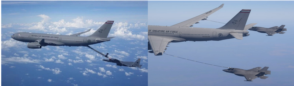
Figure 5-1: Air-to-air refuelling boom vs probe-drogue method.
