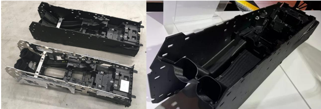
Figure 2-18: MEX manufactured centre console by BMW as published in [48]
