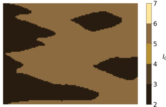
Figure 2: Topology 3 is a result of simultaneous deposition of layers including lenses.
