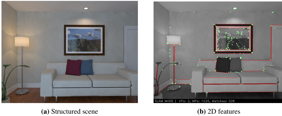
Figure 4.3: Example of point and line feature detections. Taken from [6] (Copyright © 2020, IEEE)
