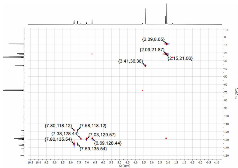
Figure S3. ^1\text{H}/^{13}\text{C} NMR HSQC spectrum of [2][\text{BArF}] in \text{THF-d}_8 at 298 K.
