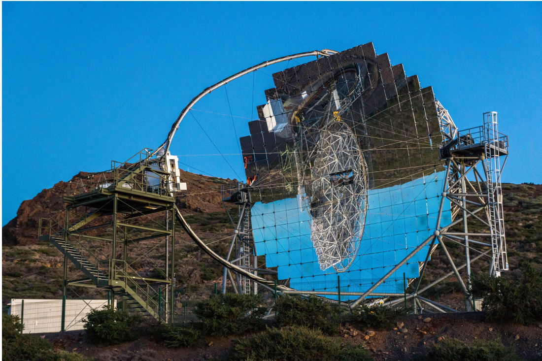
Figure 4.2: A photo of MAGIC-II. The carbon fiber structure of the main dish of MAGIC-I is seen as a reflection in the mirror. The MAGIC-II camera rests on a support beam close to the camera access tower on the left. In the center of the reflector, two mirror panels are missing. Here, several auxiliary systems are installed, such as the calibration box, the starguider camera, and the SBIG camera. See text for further information. Credit: Maximilian Linhoff
