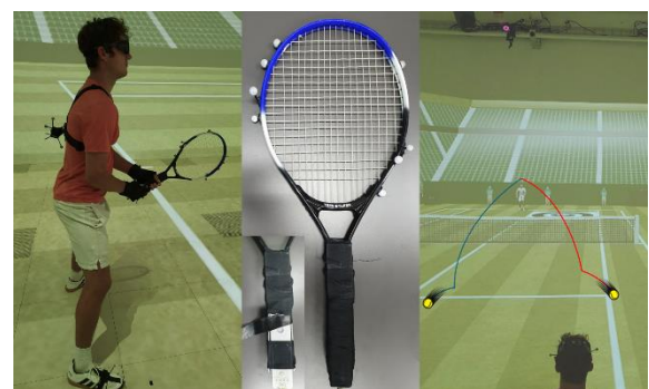
Figure 1: Setup of the virtual tennis experiment: 3D glasses, six marker clusters, a real tennis racket (with integrated Wii controller for haptic feedback), and the two possible ball trajectories (T-serve vs. wide-serve).
