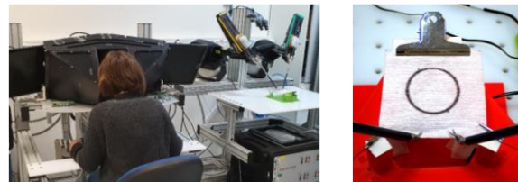
Figure 1: (a) The da Vinci Research Kit (dVRK). (b) The pattern cutting task.
