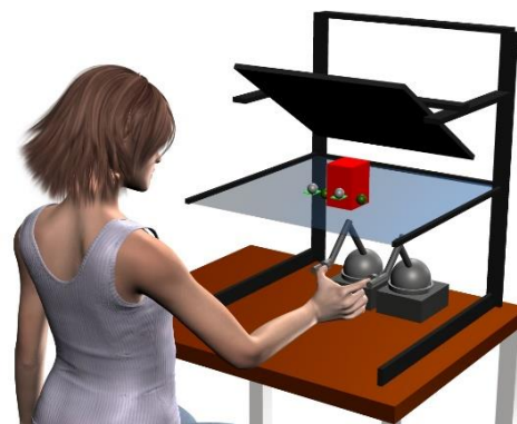
Figure 1: Virtual grasping setup consisting of two haptic robots for position and force feedback and a mirror-monitor system for visual feedback
