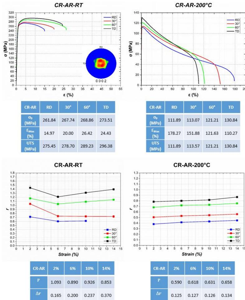
Fig. 7: Engineering stress-strain curves at RT and 200 °C of ZEWK alloy samples processed by cold rolling scheme. The measured r-values at different strains are also plotted.
