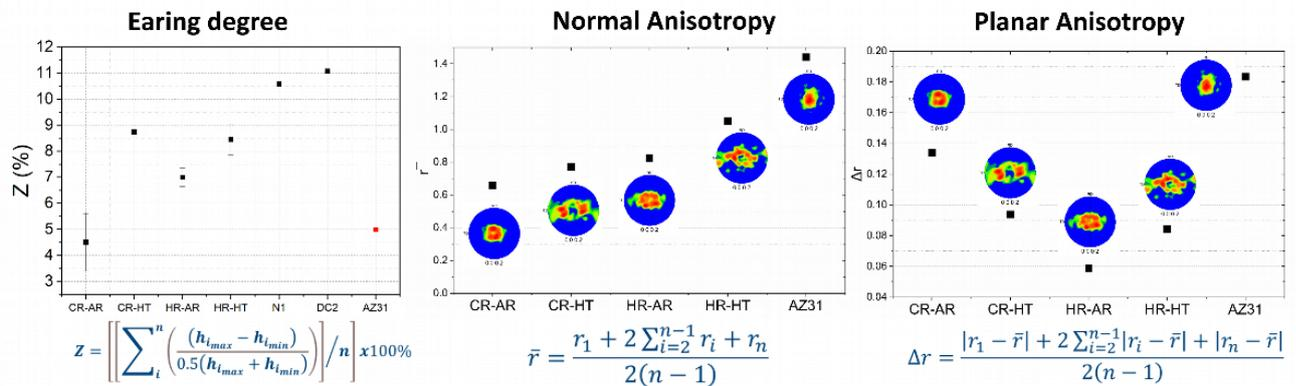
Fig. 9 presents the earing degree, the normal anisotropy and the planar anisotropy of hot-rolling, cold rolling and ECAP processed samples at 200 °C using 100 mm diameter blanks ( $DR=2$ ). The  $r_{10}$ -values obtained from tension test at 200 °C using strain rate of  $1 \times 10^{-3} \text{ s}^{-1}$ .
