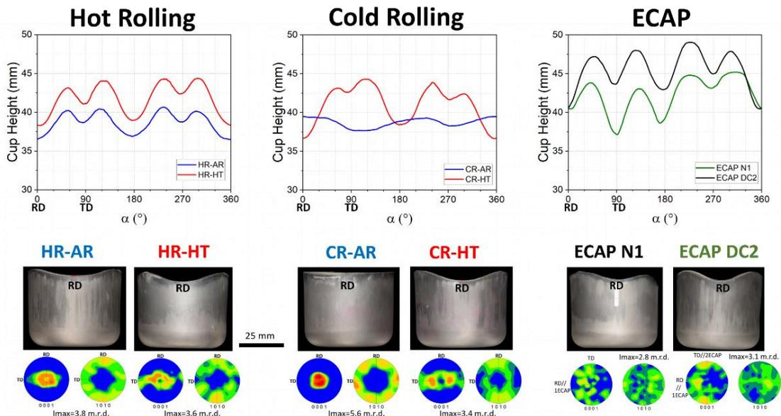
Fig. 8 presents the results of deep drawing experiments of hot-rolling, cold rolling and ECAP pro-cessed samples at 200 °C using 100 mm diameter blanks ( $DR=2$ ).
