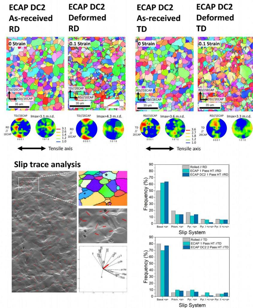
Fig. 5: Ex-situ IPF maps of RD and TD samples uniaxially deformed in tension up to 10 % strain to assess the activity of slip modes via slip trace analysis.
