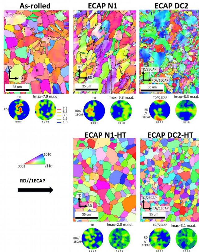
Fig. 3: Inverse pole figure (IPF) maps of a rolled sample and ECAP processed sheets following the route N1 and DC2 in as-received and annealed conditions respectively.
