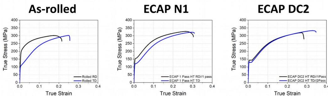
Fig. 4: True stress-true strain at RT of rolled, ECAP N1 and ECAP DC2 processed samples.
