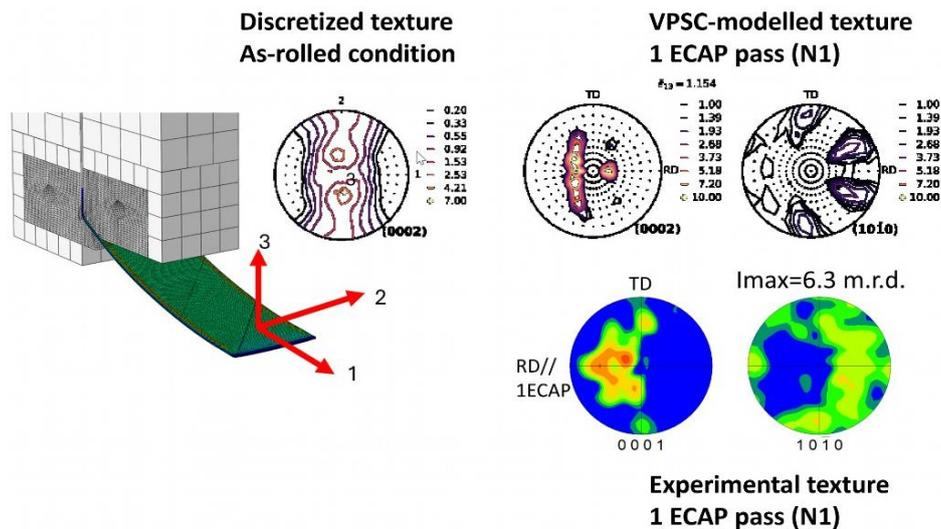
Fig. 1: FEM simulation of the ECAP process and VPSC simulated texture of the ZEWK alloy at 225 °C.
