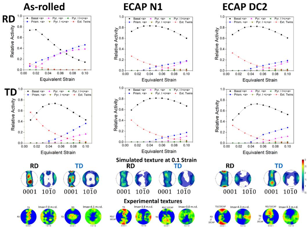
Fig. 6: VPSC modelling of as-rolled, ECAP N1 and ECAP DC2 processed samples. Exemplarily the hardening behaviour of the DC2 sample is presented. The experimental and simulated texture development are also presented.
