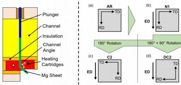
Fig. 2: Schematic representation of the ECAP tool (left) and investigated ECAP routes (right): (a) initial sheet (AR), (b) N1 route, (c) C2 route and (d) DC2 route based on [Böh23].
