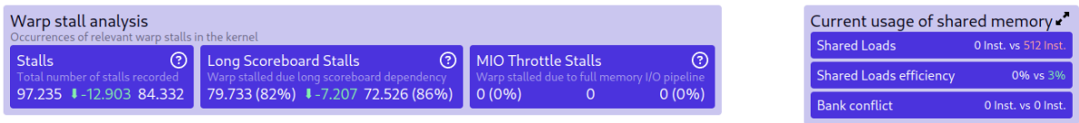
Figure 5.10.: Metrics list: Comparison after changes in Jacobi iteration kernel (Use shared analysis)
