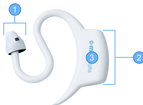
Figure 2.1: C-Med ° Alpha in-ear sensor architecture: (1) Sensor head containing the photoplethysmography (PPG) sensor and temperature sensors, (2) Preprocessing block responsible for real-time signal processing, and (3) Triaxial accelerometer for capturing motion data, adapted from [17].
