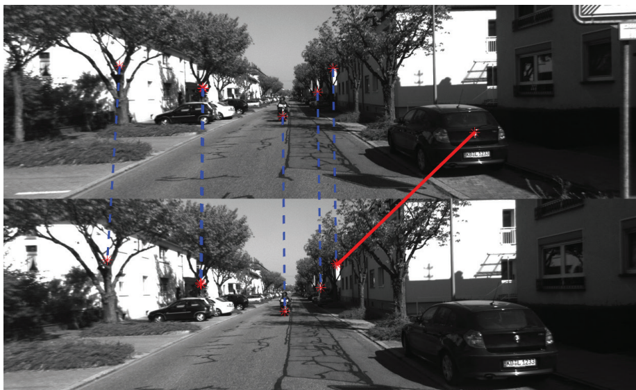
FIGURE 5 An example of wrong association and outlier features; images from public data set (Geiger et al., 2012)
