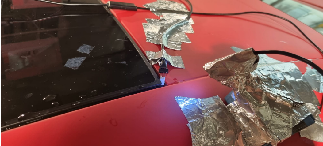
(a) Humidity sensor and endoscope installation
