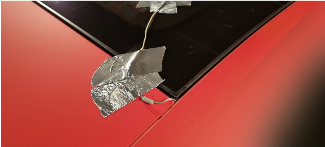
(b) Water temperature sensor installation
