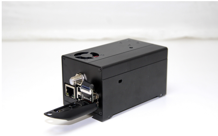
Figure 2.3: Tower Motion Module prototype consisting of a single-board computer, an acceleration element, an RTK module with antenna connector, and external memory for data logging.
