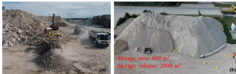
Figure 1: Manufacture (a) and storage (b) of RA on the Valosphère recycling platform in France.
