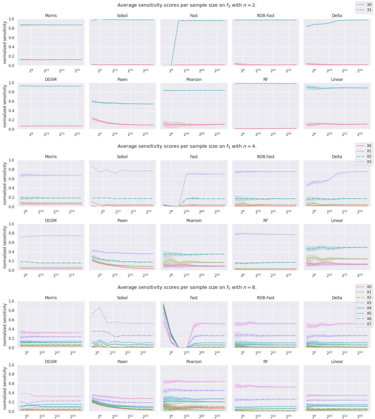
FIGURE 10. Sensitivity analysis on f_3 in 2, 4 and 8 dimensions. Each plot shows the results using a different algorithm. The sample size is on the x-axis and the scaled sensitivity on the y-axis. The shaded area denotes the standard deviation from the 10 runs with different random seed.
