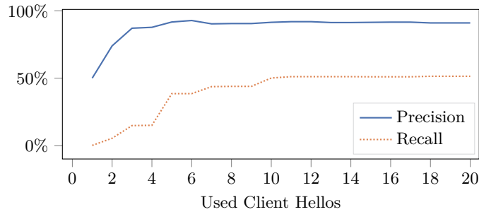
Figure 2.6: Influence of the CHs on the C2 detection with an 80% threshold ( cf. , Sosnowski et al. [8]).
