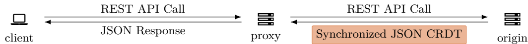
Figure 4.1: Example client server architecture utilizing CWC for a REST API transmitting JSON.
