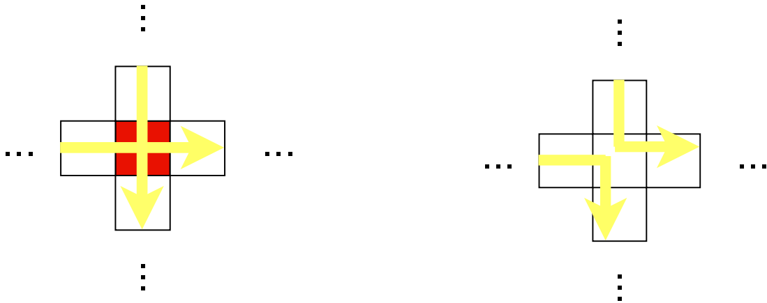
(a) This is an example of the crossing in the grained routing. The red-filled rectangle is where the crossing happens.
