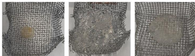
Figure S30: Images of hydrogel samples obtained from functionalized polymers: hydrogel in the dry state (left), highly swollen hydrogel without structural integrity (Table 2, Entry 9) (middle) and swollen hydrogel forming a soft and brittle chip (Table 2, Entry 11).
