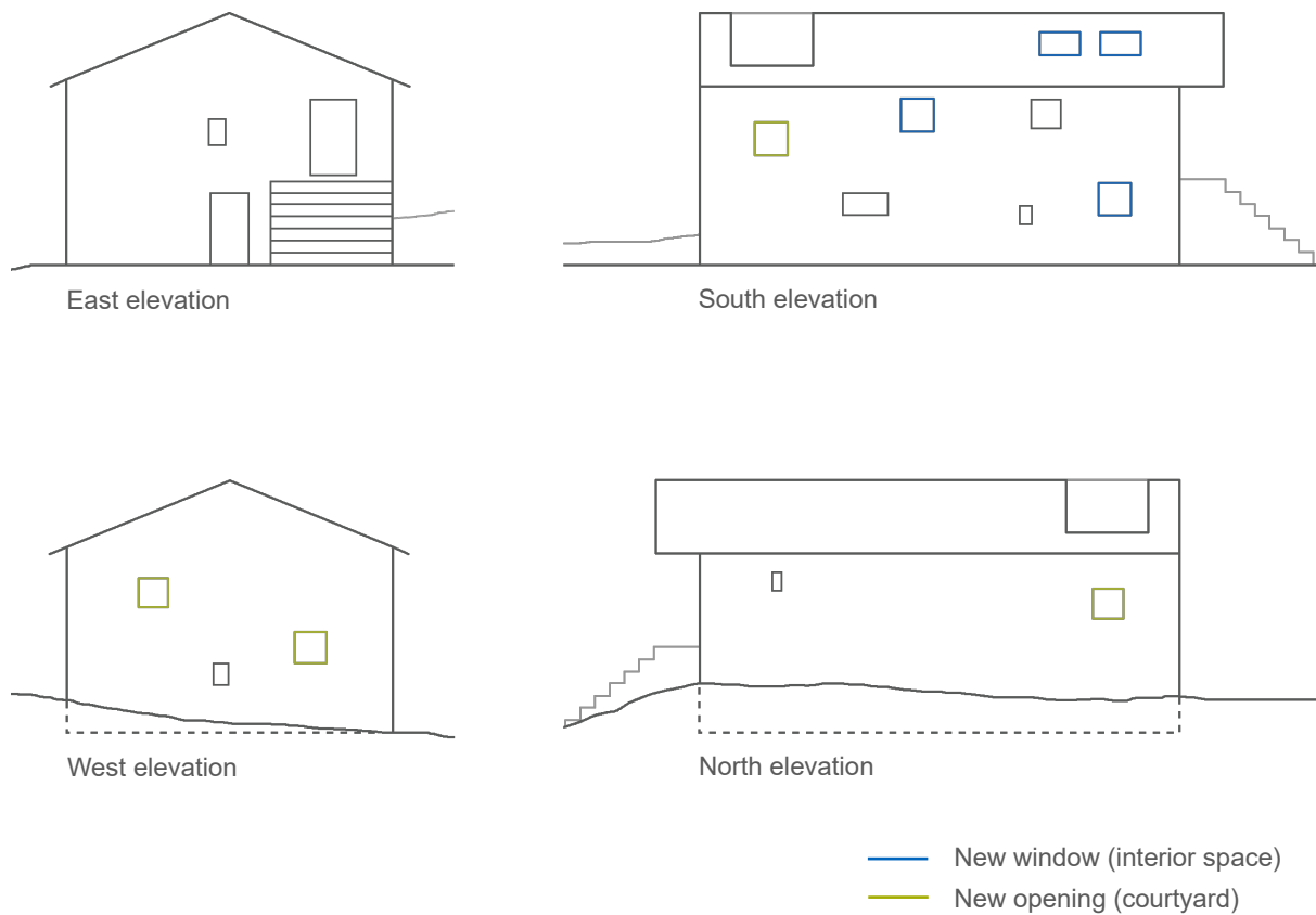
Figure 43: Scheme of existing and planned new openings
