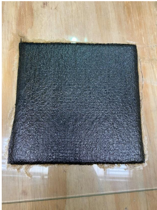
Fig.A- 23: TA/ELO 1.5 CF composite plate manufactured with UD SGL fabric and vacuum bagging
