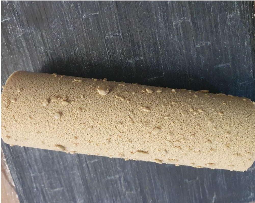
Fig.A- 6: TA agglomerates on the sponge roller during lamination
