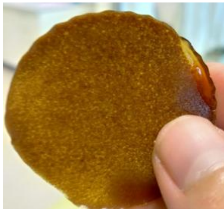
Fig.A- 11: Inhomogeneous TA/ELO sample after curing at 120 °C
