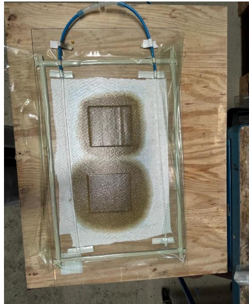
Figure 52: Example of TA/ELO CF composites plates after curing manufactured with UD SGL fabric or towpregs and vacuum bagging technique.
