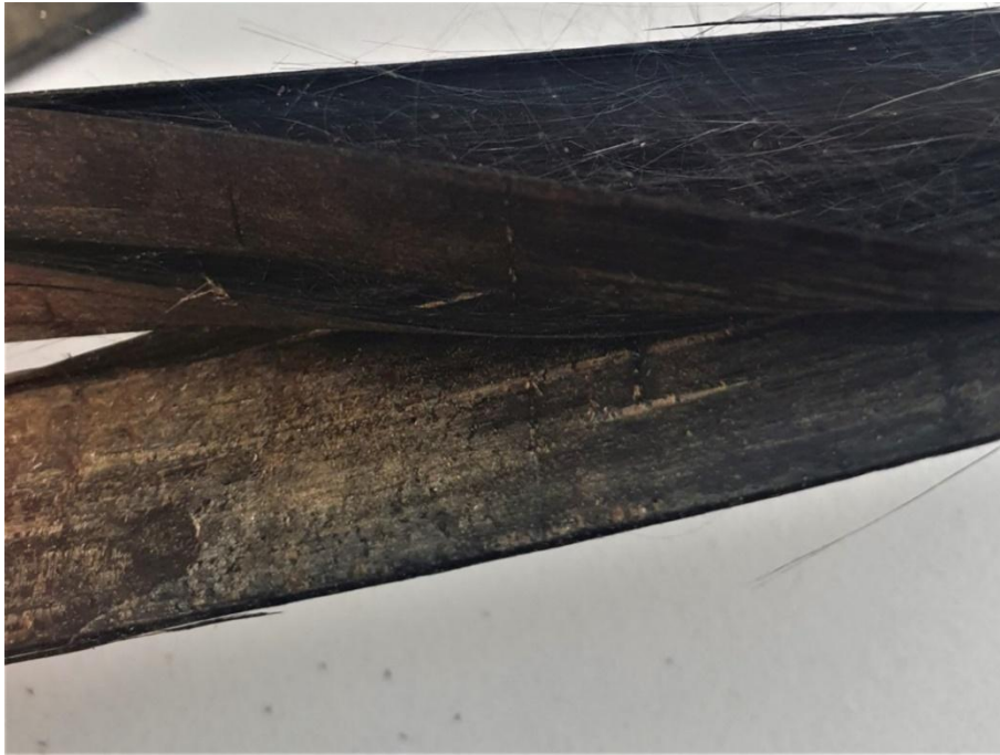
Figure 47: TA particles and dry spots in the TA/ELO composites. Sample after flexural testing.
