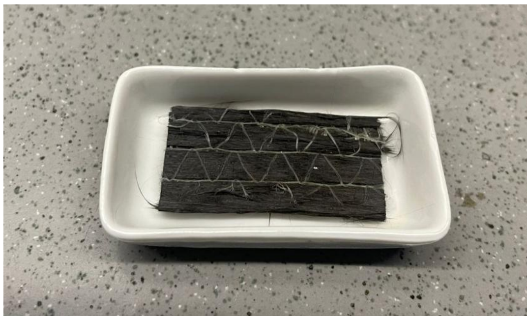
Fig.A- 25: TA/ELO composite with stitched UD-CF fabric after immersion in NaOH solution, washing in water and drying. Recovery of the CF.
