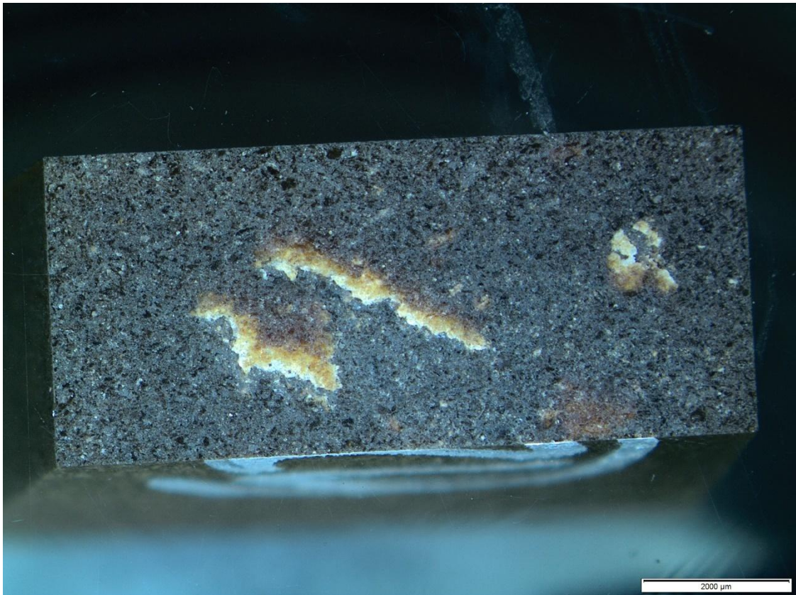
Figure 41: Microscopy image of TA/ELO 2.0 recycled at 145 °C for 2 h. Length of the scale: 2000 μm.
