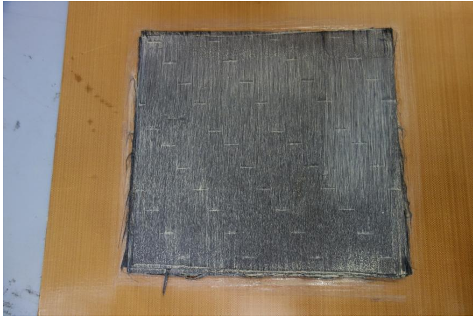
Fig.A- 8: 3/1 twill UD CF fabrics stacked on each other after being hand-laminated.
