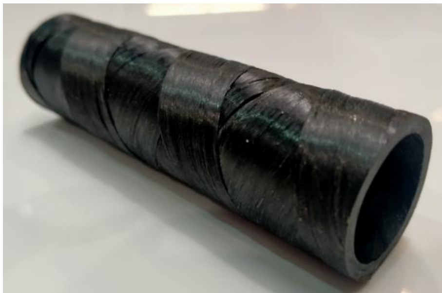
Figure 60: Pipe made with TA/ELO-CF towpregs winded on a metal mandrel.
