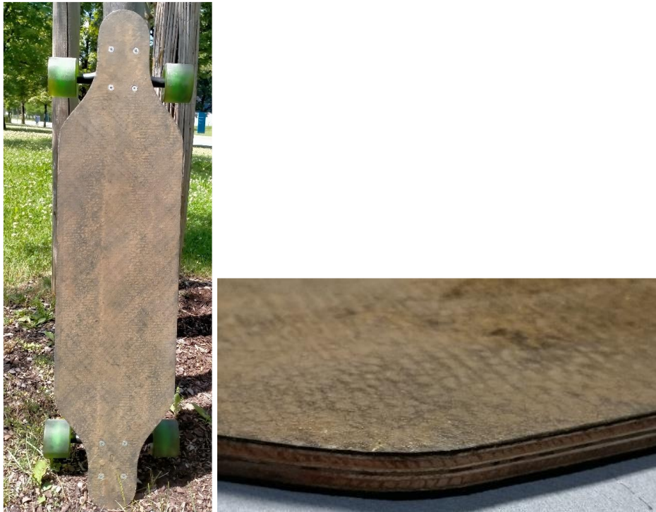
Figure 59: Longboard made with a plywood core, CF fabrics and TA/ELO.
