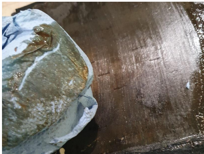
Fig.A- 9: Oily surface on TA/ELO CF composites plates after hot-pressing.
