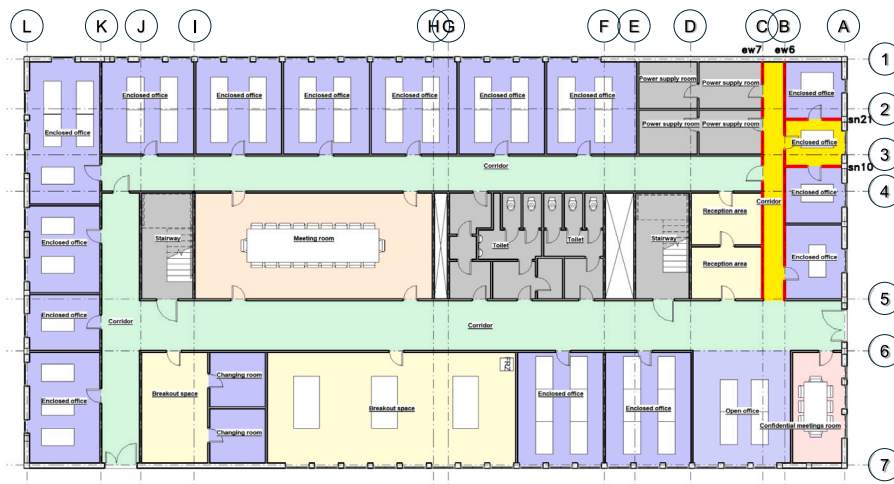
Fig. 7. Propagation results showcasing with one single propagation (IBC 1020.2, IBC 1207.1, and IBC 1207.3). Spaces subject to propagation are highlighted in yellow, while affected objects are marked in red. The walls associated with ew_6 , sn_{21} and sn_{10} are identified for potential local variation. Conversely, the wall of the service space, denoted by ew_7 , is designated to remain unchanged from the initial design.
