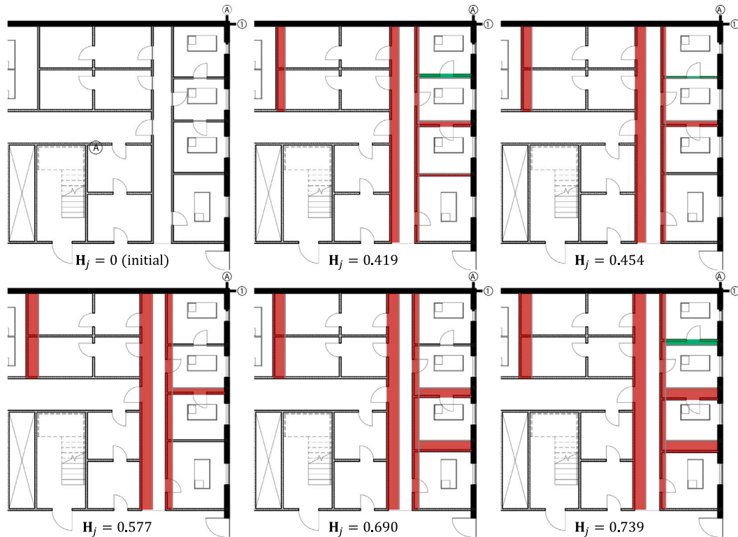
Fig. 12. Comparison of valid design alternatives across a diverse range of H_j , from the identified smallest to largest values. Initial wall locations are shaded in grey, with red indicating wall movement in a further direction and green indicating movement in a closer direction, relative to reference grids 1 and A.
