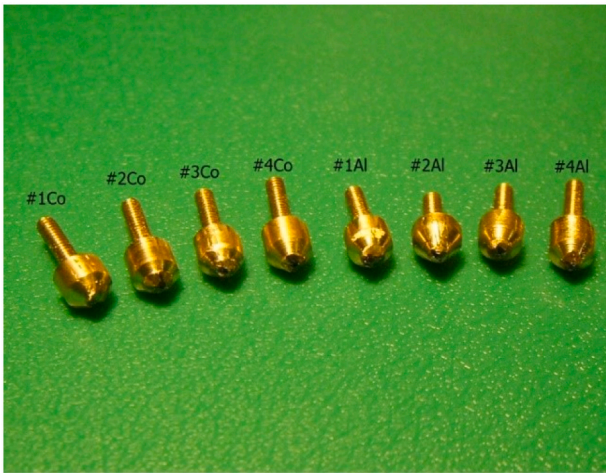
Fig. 6. Four probes with diamonds synthesized in Fe-Co-C-B growth system (#Co, #2Co, #3Co, #4Co) and four probes synthesized in Fe-Al-C-B growth system (#1Al, #2Al, #3Al, #4Al).
