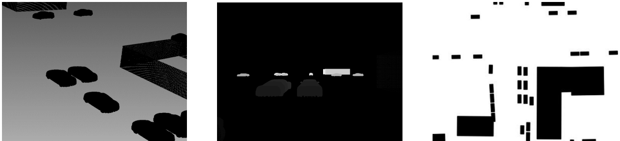
FIGURE 2: Visualization of the three-dimensional point cloud surrounding the observer under investigation (left), the corresponding depth image captured by the front camera (center), and the BEV representation of the same scene utilized for the NN approach (right).
