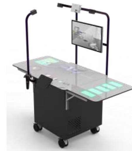
Teleoperation cell: GUI + movement tracking controller /haptic controller
